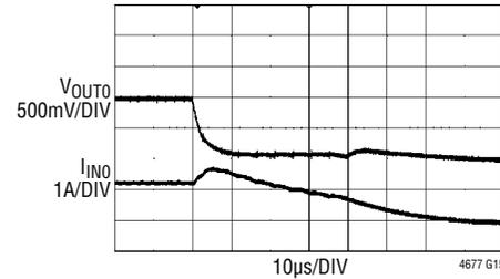
FIGURE 56 CIRCUIT AT  $12\text{V}_{\text{IN}}$ , 18A LOAD ON
