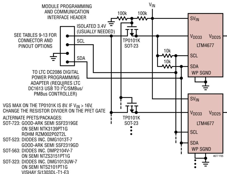
**Figure 5. Circuit Suitable for Programming EEPROM/NVM of LTM4677 and Other ADI PSM Modules/ICs in Vast Systems, Even When V<sub>IN</sub> Power is Absent, 0°C < T<sub>J</sub> ≤ 85°C**
