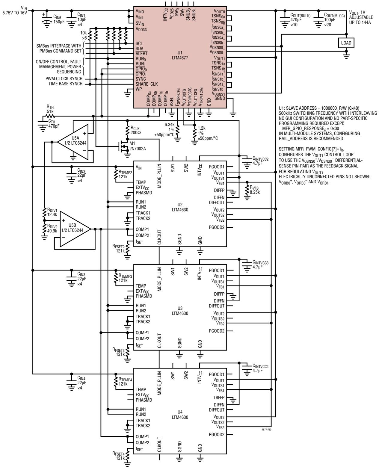
Figure 30. One LTM4677 Operating In Parallel with 3xLTM4630A Producing 1V<sub>OUT</sub> at up to 144A. Power System Management Features Accessible Through LTM4677 Over 2-Wire I<sup>2</sup>C/SMBus/PMBus Serial Interface.
