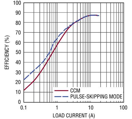
**Dual Phase Single Output Efficiency,  $5V_{IN}$ ,  $V_{IN} = SV_{IN} = INTV_{CC} = 5V$ ,  $V_{OUT0}$  and  $V_{OUT1}$  Paralleled CCM Mode**
