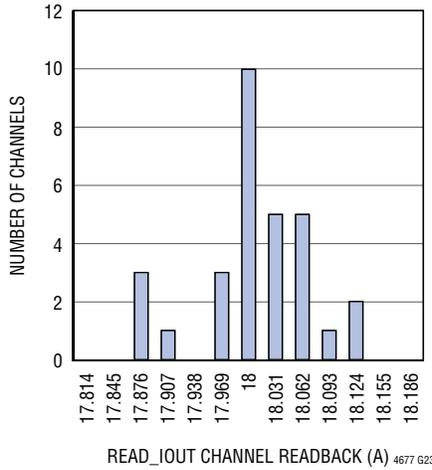
**READ\_IOUT of 30 LTM4677 Channels (DC2066A)  $12\text{V}_{\text{IN}}$ ,  $1\text{V}_{\text{OUT}}$ ,  $T_J = 125^\circ\text{C}$ ,  $I_{\text{OUT}n} = 18\text{A}$ , System Having Reached Thermally Steady-State Condition, No Airflow**
