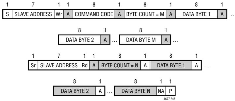
**Figure 46. Block Write – Block Read Process Call**
