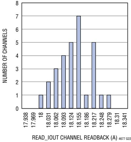
**READ\_IOUT of 30 LTM4677 Channels (DC2066A)  $12\text{V}_{\text{IN}}$ ,  $1\text{V}_{\text{OUT}}$ ,  $T_J = 25^\circ\text{C}$ ,  $I_{\text{OUT}n} = 18\text{A}$ , System Having Reached Thermally Steady-State Condition, No Airflow**
