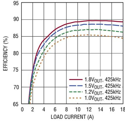
**Single Output Pulse-Skipping Efficiency,  $V_{IN} = SV_{IN} = 12V$ ,  $INTV_{CC}$  Open,  $12V_{IN}$  to  $1.5V_{OUT}$ , 425kHz**
