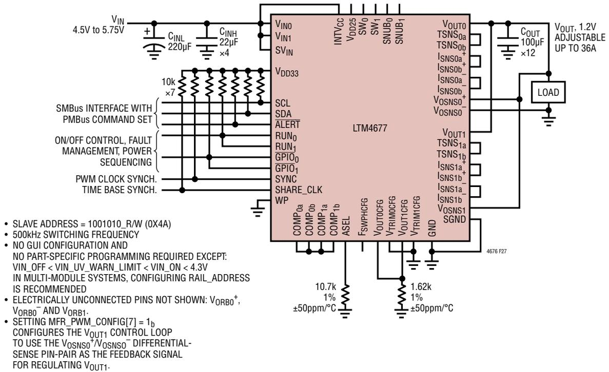
Figure 27. 36A, 1.2V Output DC/DC µModule Regulator with I<sup>2</sup>C/SMBus/PMBus Serial Interface
