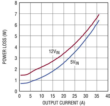
Figure 12. 1.2V<sub>OUT</sub> Power Loss Curve
