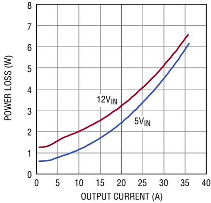
Figure 11. 0.9V<sub>OUT</sub> Power Loss Curve
