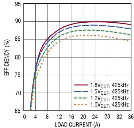
**TYPICAL PERFORMANCE CHARACTERISTICS**  $T_A = 25^\circ\text{C}$ ,  $12\text{V}_{\text{IN}}$  to  $1\text{V}_{\text{OUT}}$ , unless otherwise noted.
