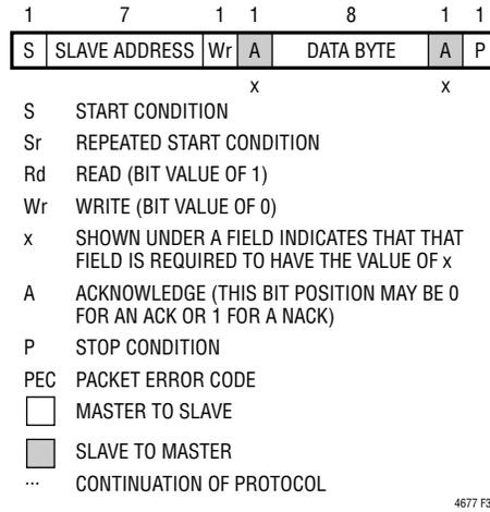
Figure 32. PMBus Packet Protocol Diagram Element Key
