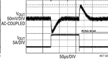
FIGURE 56 CIRCUIT AT  $12\text{V}_{\text{IN}}$ ,  $\text{INTV}_{\text{CC}}$  OPEN
