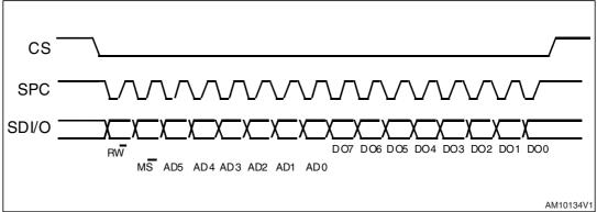
The SPI read command is performed with 16 clock pulses:
