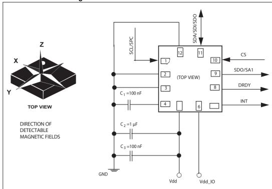
Figure 5. LIS3MDL electrical connections
