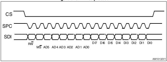
The SPI Write command is performed with 16 clock pulses. A multiple byte write command is performed by adding blocks of 8 clock pulses to the previous one.
