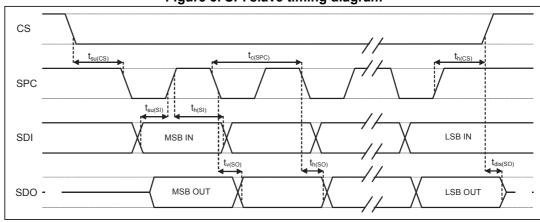
Figure 3. SPI slave timing diagram
