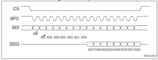
The SPI read command is performed with 16 clock pulses. A multiple byte read command is performed by adding blocks of 8 clock pulses to the previous one.
