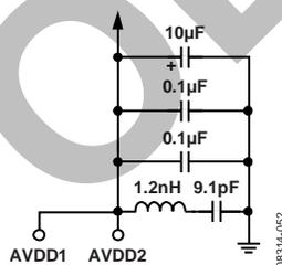
Figure 56. GSM Filter on the Analog Supply Pins
