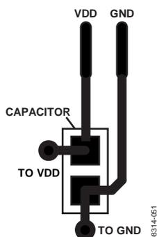
Figure 55. Recommended Power Supply Bypass Capacitor Layout
