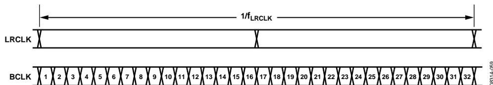
Figure 63. Example: 32 BCLK Cycles per Frame
