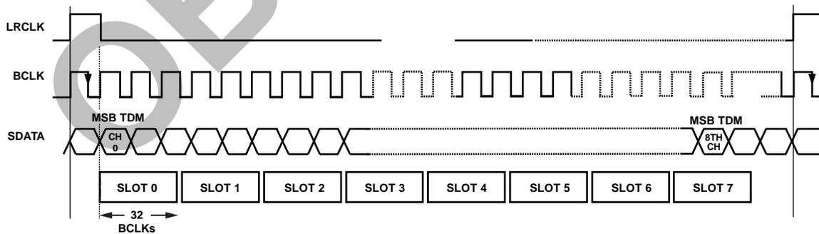
Figure 50. TDM Mode with Pulse Word Clock
