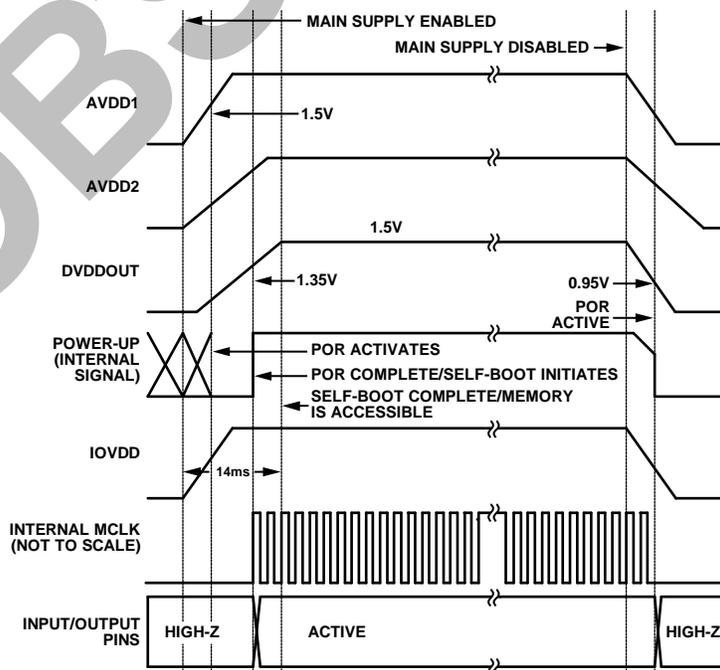
Figure 27. Power-Up and Power-Down Sequence Timing Diagram
