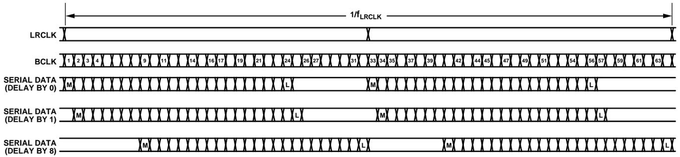
Figure 68. Serial Audio Data Delay Example Settings
