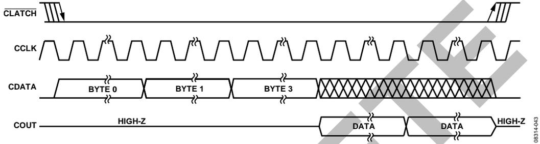
Figure 44. SPI Read from ADAU1781 Clocking (Single-Read Mode)
