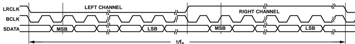
Figure 46. I²S Mode—16 Bits to 24 Bits per Channel
