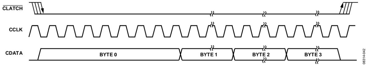
Figure 43. SPI Write to ADAU1781 Clocking (Single-Write Mode)
