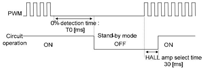
Figure 23. Stand-by mode and quick start function
