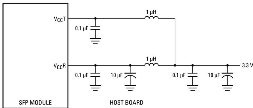
NOTE: INDUCTORS MUST HAVE LESS THAN 1 Ω SERIES RESISTANCE PER MSA.
