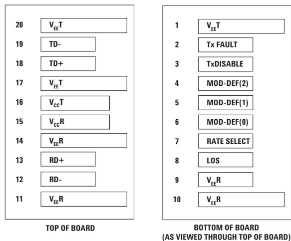
Figure 2. Connection Diagram of Module Printed Circuit Board
