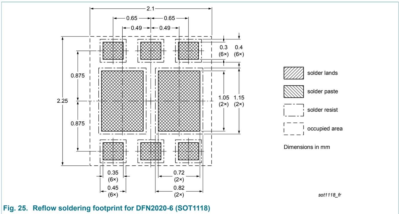
Fig. 25. Reflow soldering footprint for DFN2020-6 (SOT1118)
