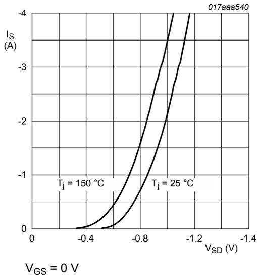
Fig. 18. MOSFET transistor: Source current as a function of source-drain voltage; typical values
