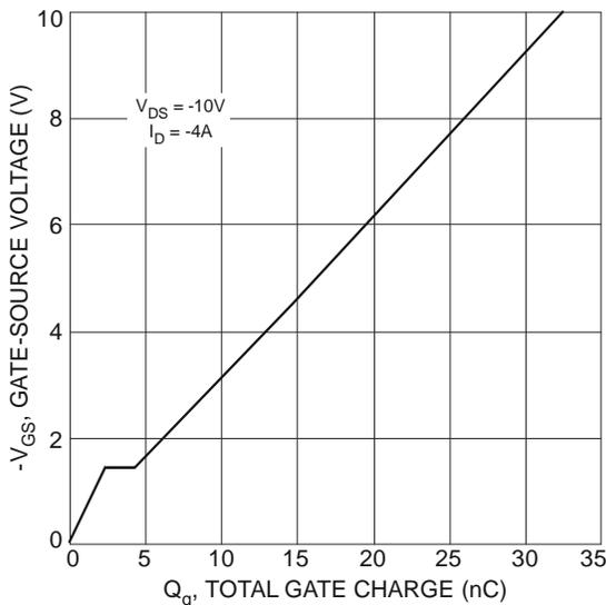
Fig. 22 Gate-Source Voltage vs. Total Gate Charge
