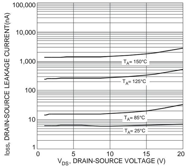
Fig. 10 Typical Drain-Source Leakage Current vs. Drain-Source Voltage
