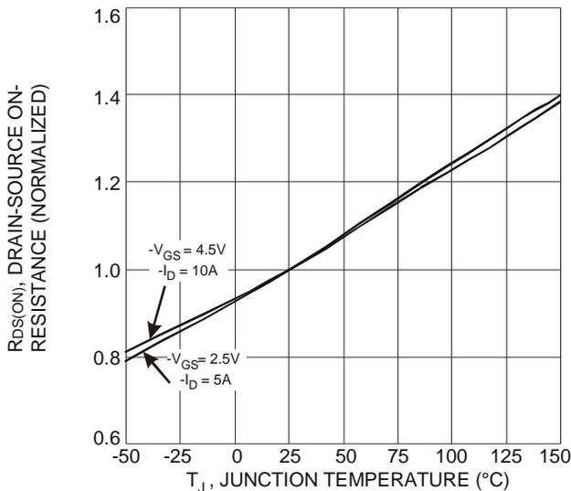
Fig. 16 On-Resistance Variation with Temperature
