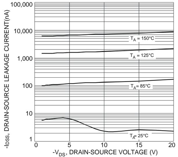
Fig. 21 Typical Drain-Source Leakage Current vs. Drain-Source Voltage
