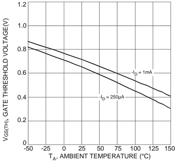
Fig. 18 Gate Threshold Variation vs. Ambient Temperature
