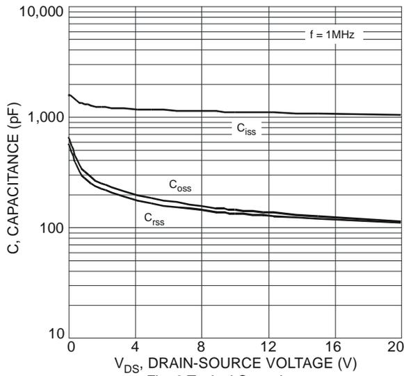
Fig. 9 Typical Capacitance
