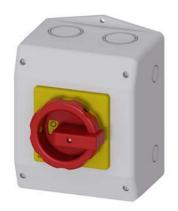
SENTRON, Switch disconnector 3LD, emergency switching-off switch, 3-pole, Iu: 63 A, operating power / at AC-23 A 400 V: 22 kW, Molded plastic encapsulation for inch cable gland, rotary operating mechanism, red/yellow
