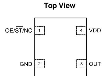
**Figure 1. Pin Assignments**
