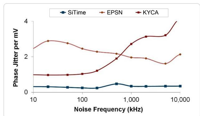
Figure 4. Power Supply Noise Rejection<sup>[4]</sup>
