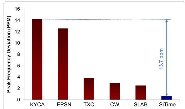
Figure 6. Shock Robustness<sup>[6]</sup>
