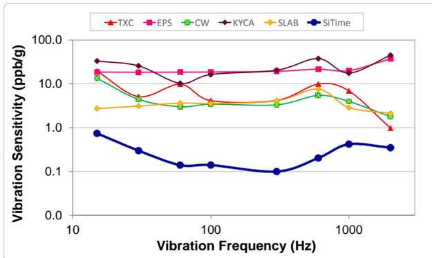
Figure 5. Vibration Robustness<sup>[5]</sup>
