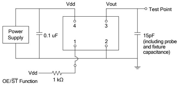
Figure 2. Test Circuit
