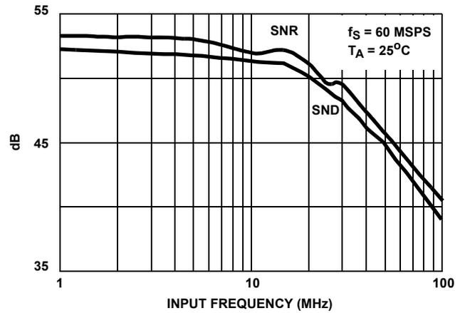
FIGURE 4. SINAD AND SNR vs INPUT FREQUENCY
