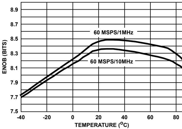
FIGURE 15. EFFECTIVE NUMBER OF BITS (ENOB) vs TEMPERATURE
