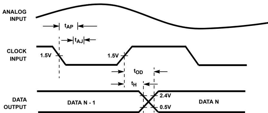
**FIGURE 2. INPUT-TO-OUTPUT TIMING**
