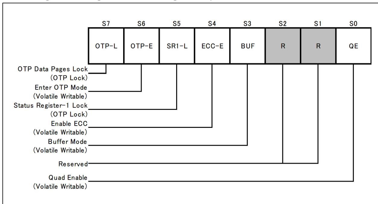
Figure 7-2 Configuration Register / Status Register-2 (Address Bxh)
