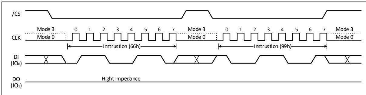
Figure 8-2 Device Reset Instruction (66h+99h)
