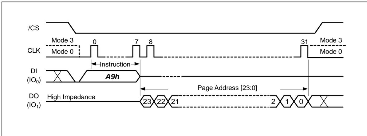
Figure 8-11 Last ECC Failure Page Address Instruction
