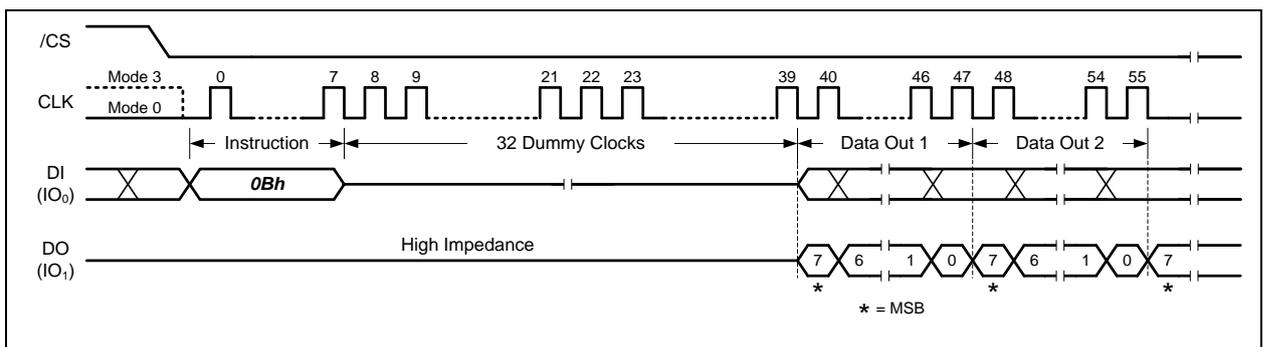
Figure 8-22 Fast Read Instruction (Continuous Read Mode, BUF=0)
