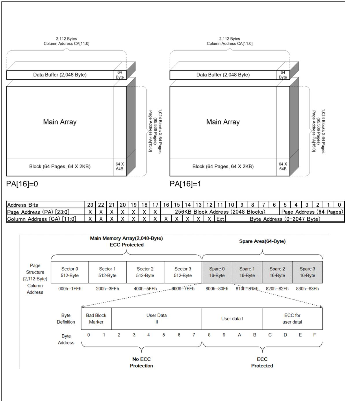
Figure 5-1 W25N02JW Flash Memory Architecture and Addressing
