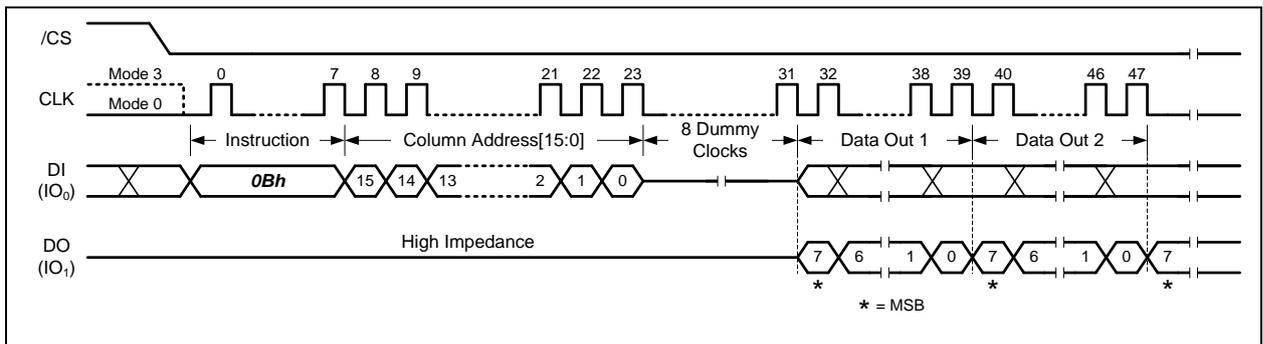
Figure 8-21 Fast Read Instruction (Buffer Read Mode, BUF=1)
