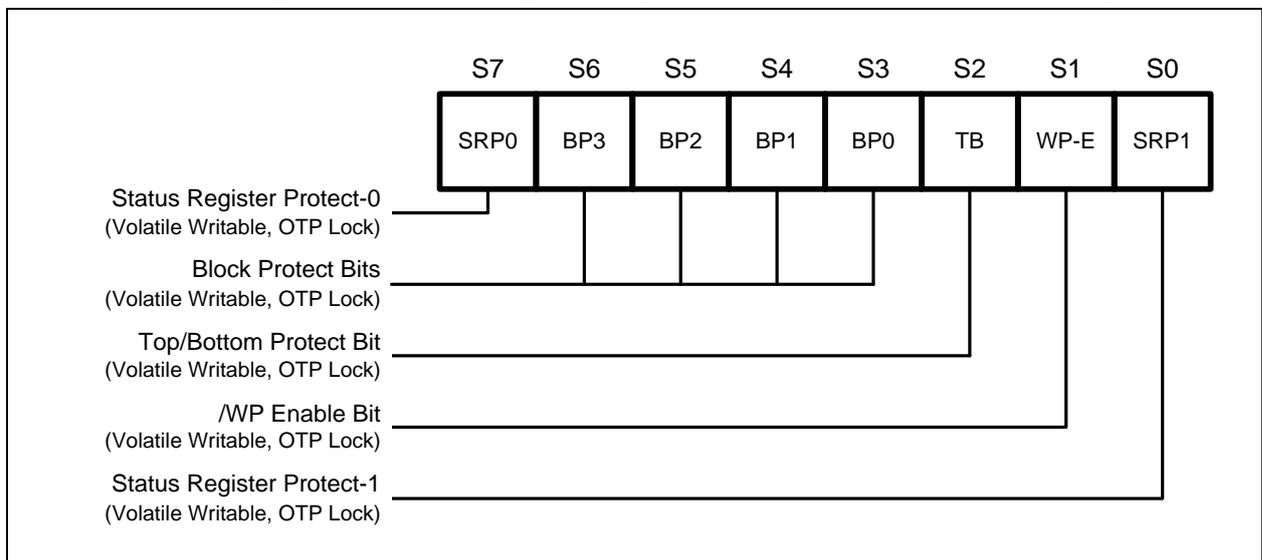
Figure 7-1 Protection Register / Status Register-1 (Address Axh)
