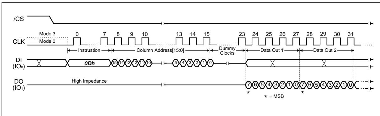
Figure 8-41 DTR Fast Read Instruction (Buffer Read Mode, BUF=1)
