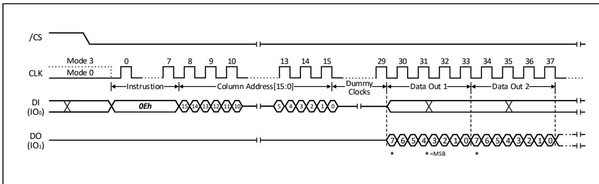
Figure 8-43 DTR Fast Read with 4-Byte Address Instruction (Buffer Read Mode, BUF=1)
