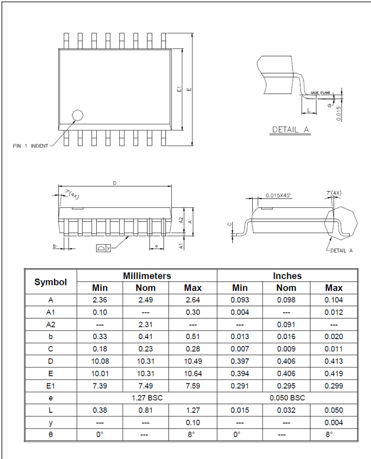
Figure 11-2 16-Pin SOIC 300mil (Package Code SF)
