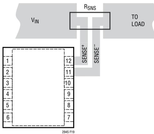
Figure 19. Recommended Layout for Kelvin Connection
