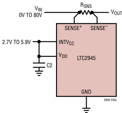
(c) Power from Low Voltage Secondary Supply
