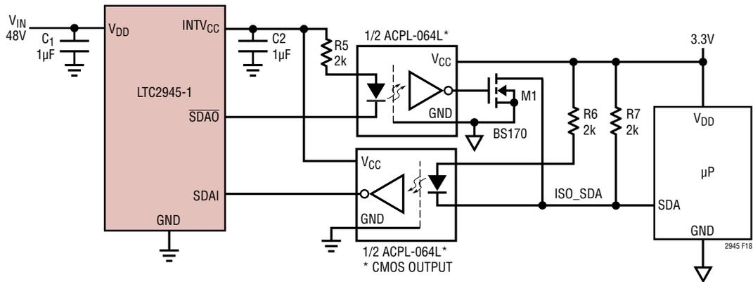
Figure 18. Opto-Isolation of I<sup>2</sup>C Interface with Low Power, High Speed Opto-Couplers (SCL Omitted for Clarity)
