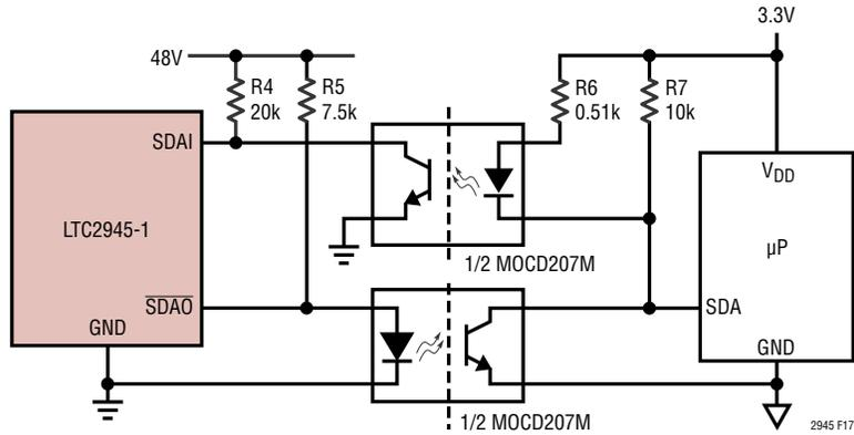
Figure 17. Opto-Isolation of a 1.5kHz I<sup>2</sup>C Interface Between LTC2945-1 and Microcontroller (SCL Omitted for Clarity)
