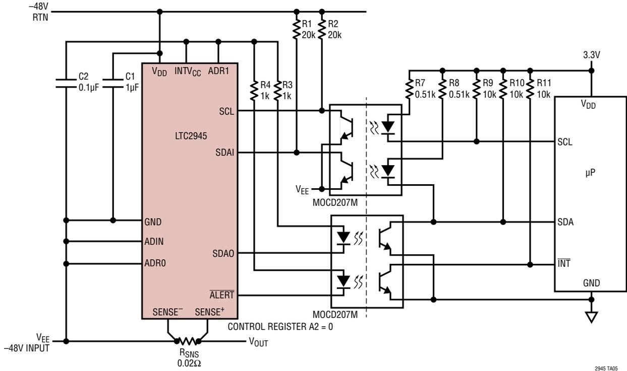
Power Monitoring in -48V Harsh Environment Using INTV<sub>CC</sub> Shunt Regulator to Tolerate 200V Transients
