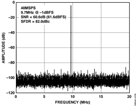
Figure 20. AD9609-40 Single-Tone FFT with  $f_{IN} = 9.7$  MHz
