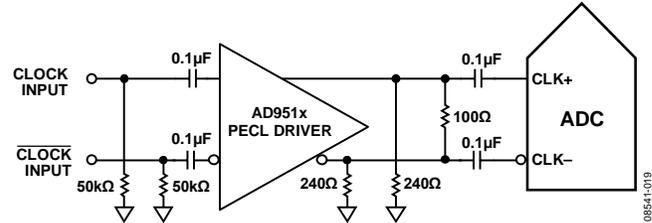
Figure 48. Differential PECL Sample Clock (Up to 625 MHz)
