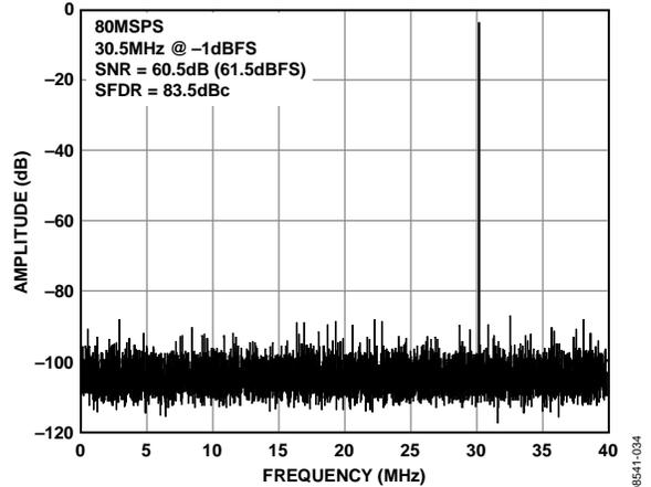
Figure 7. AD9609-80 Single-Tone FFT with  $f_{IN} = 30.5$  MHz
