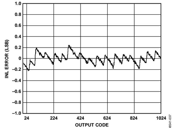
Figure 14. INL with  $f_{IN} = 9.7$  MHz
