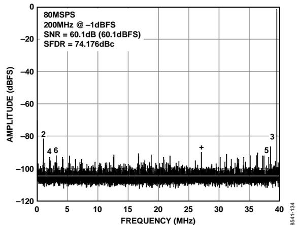
Figure 8. AD9609-80 Single-Tone FFT with  $f_{IN} = 200$  MHz
