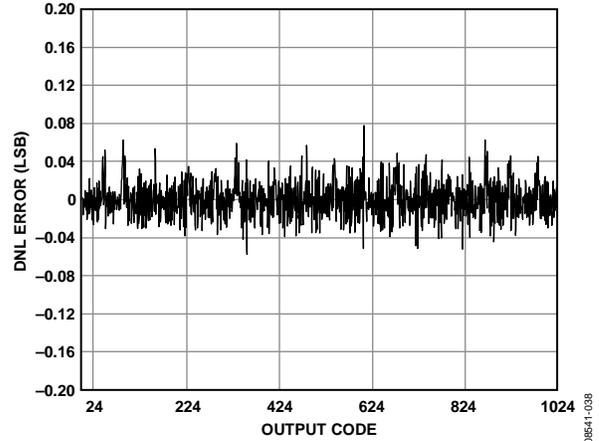
Figure 13. DNL Error with  $f_{IN} = 9.7$  MHz
