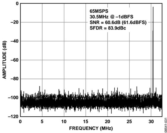
Figure 17. AD9609-65 Single-Tone FFT with  $f_{IN} = 30.5$  MHz
