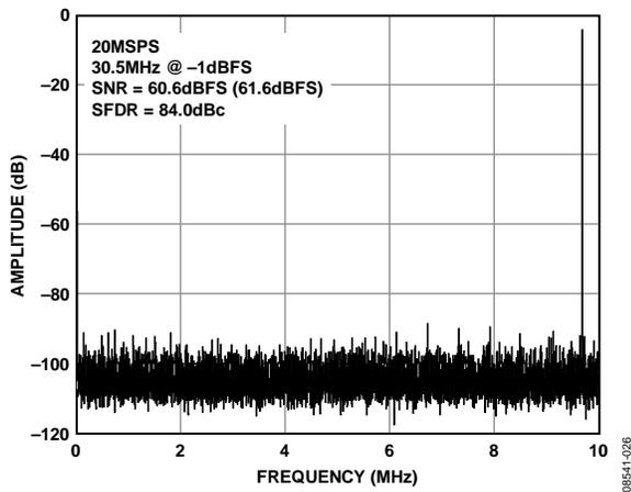
Figure 24. AD9609-20 Single-Tone FFT with  $f_{IN} = 30.5$  MHz
