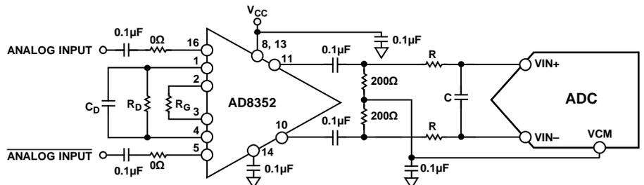
Figure 41. Differential Input Configuration Using the AD8352
