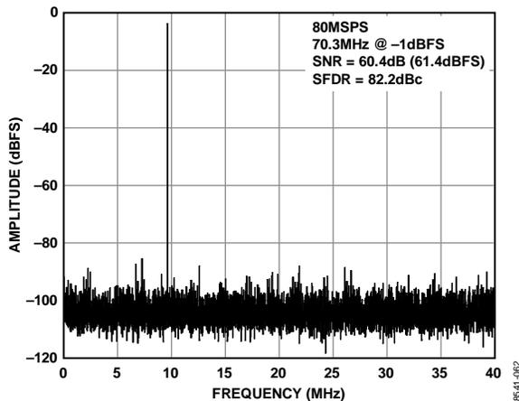
Figure 5. AD9609-80 Single-Tone FFT with  $f_{IN} = 70.3$  MHz
