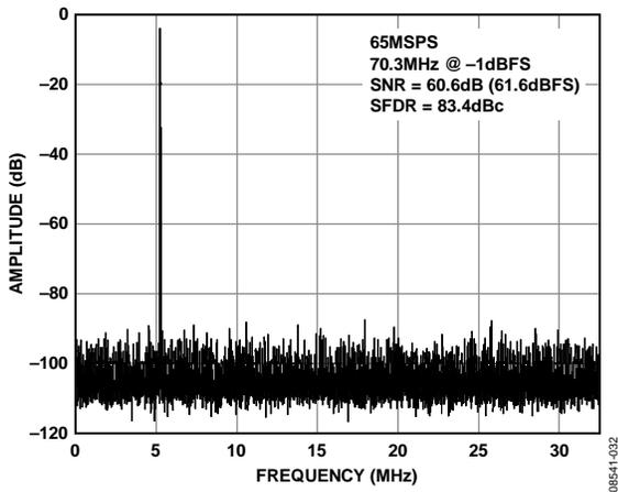
Figure 16. AD9609-65 Single-Tone FFT with  $f_{IN} = 70.3$  MHz
