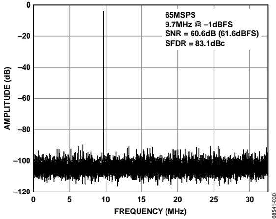
Figure 15. AD9609-65 Single-Tone FFT with  $f_{IN} = 9.7$  MHz
