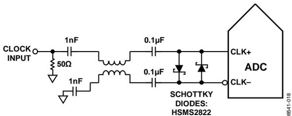
Figure 47. Balun-Coupled Differential Clock (Up to 625 MHz)
