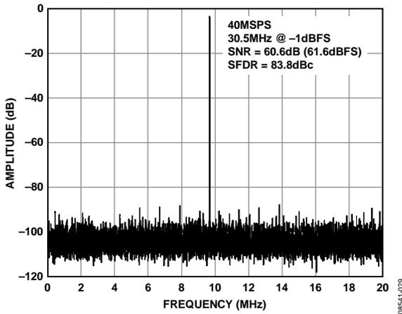
Figure 21. AD9609-40 Single-Tone FFT with  $f_{IN} = 30.5$  MHz
