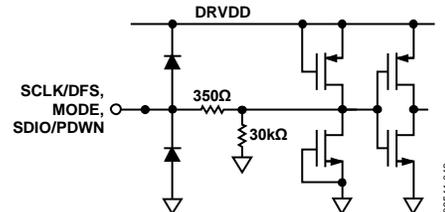
Figure 31. Equivalent SCLK/DFS, MODE, and SDIO/PDWN Input Circuit
