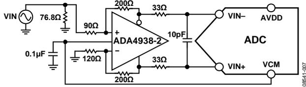
Figure 37. Differential Input Configuration Using the ADA4938-2
