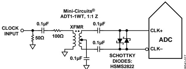
Figure 46. Transformer-Coupled Differential Clock (Up to 200 MHz)
