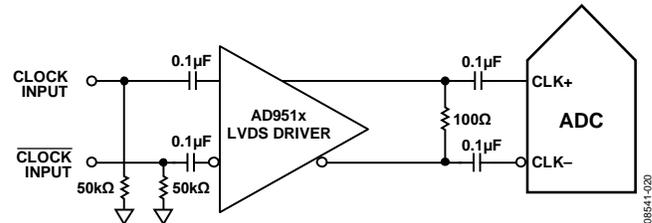
Figure 49. Differential LVDS Sample Clock (Up to 625 MHz)
