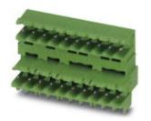
Header, Nominal current: 10 A, Rated voltage (III/2): 320 V, Number of positions: 9, Pitch: 5 mm, Color: green, Contact surface: Tin, Mounting: Wave soldering, The article can be aligned to create different nos. of positions! In combination with MVSTB or FKCV plug components, both an MVSTBW (or FKCVW) and an MVSTBR plug (or FKCVR) must be used. Combination with TMSTBP plug components is not possible!
