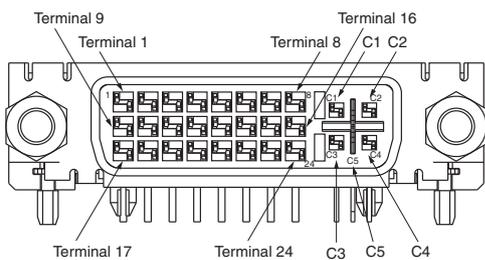
Note: The digital type does not have C1 to C5.
