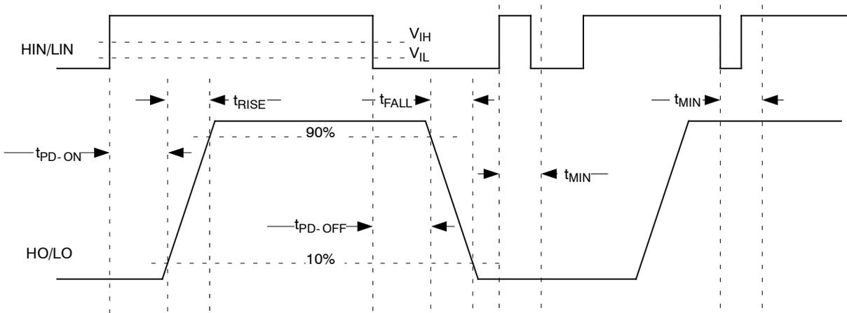
Figure 3. Propagation Delay, Rise and Fall Time
