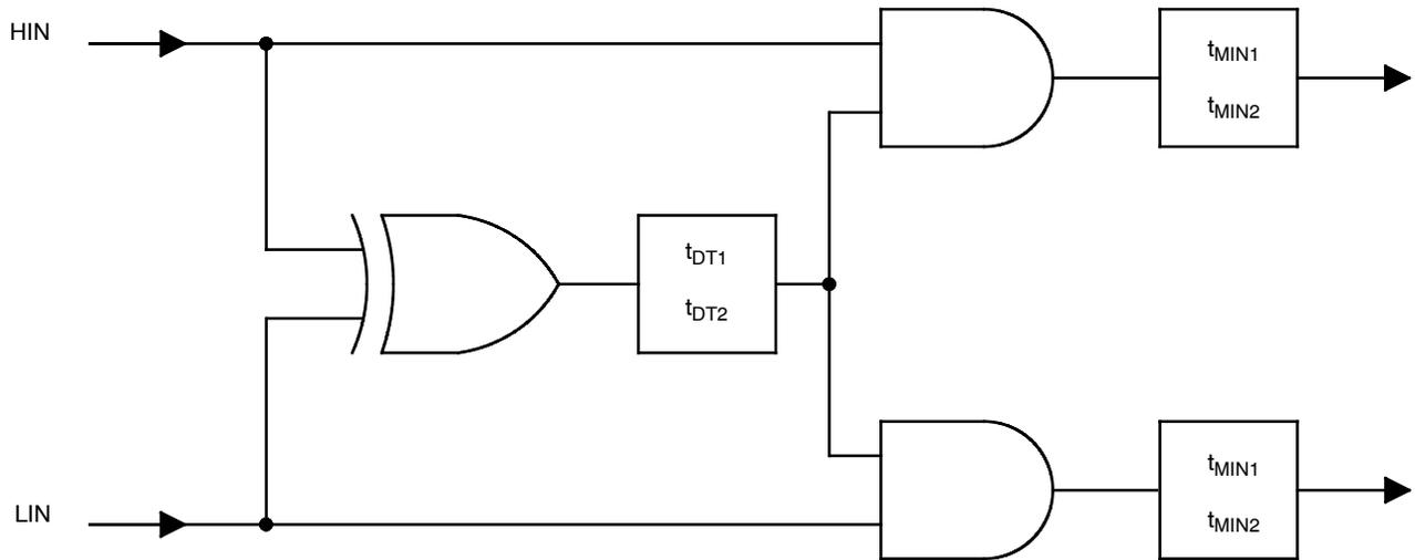
Figure 7. Input Circuit
