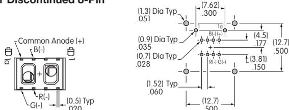
Terminal Detail & Footprint for Replacement 4-Pin
