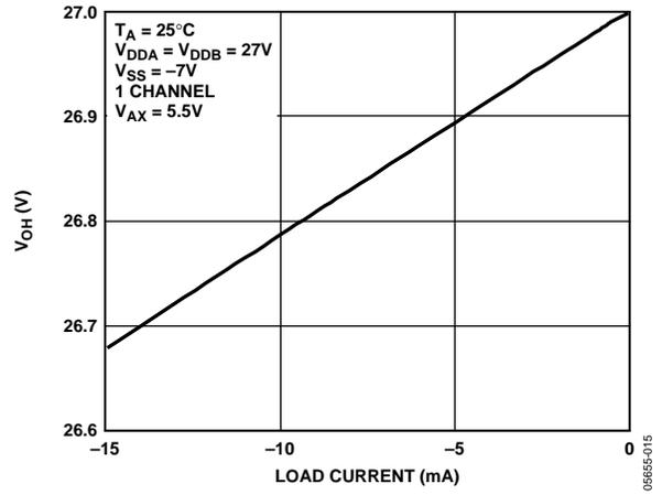
Figure 17. Output Voltage ( $V_{OH}$ ) vs. Load Current
