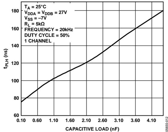
Figure 12. Propagation Delay ( $t_{PLH}$ ) vs. Capacitive Load
