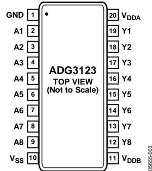
Figure 3. Pin Configuration
