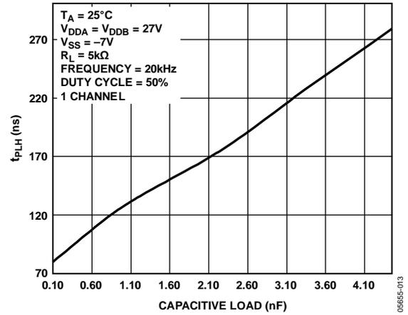
Figure 13. Propagation Delay ( $t_{PLH}$ ) vs. Capacitive Load
