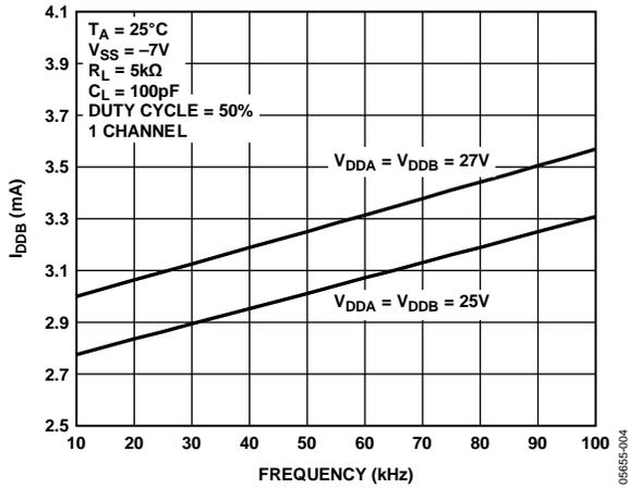
Figure 4. Supply Current ( $I_{DDB}$ ) vs. Frequency
