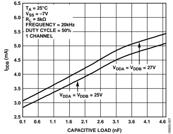
Figure 7. Supply Current ( $I_{DDB}$ ) vs. Capacitive Load
