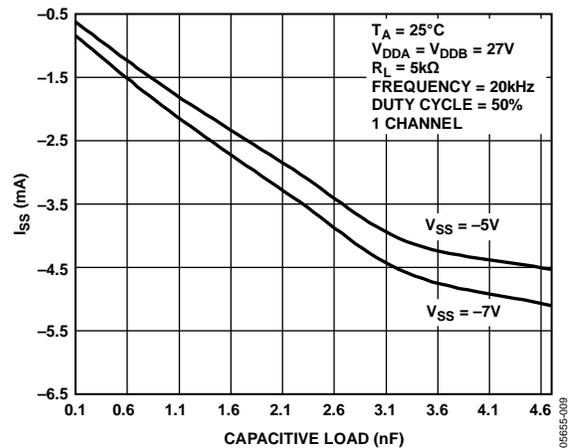
Figure 9. Supply Current ( $I_{SS}$ ) vs. Capacitive Load
