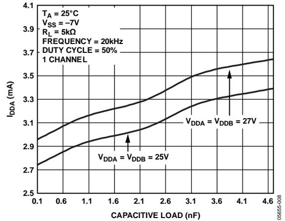
Figure 8. Supply Current ( $I_{DDA}$ ) vs. Capacitive Load
