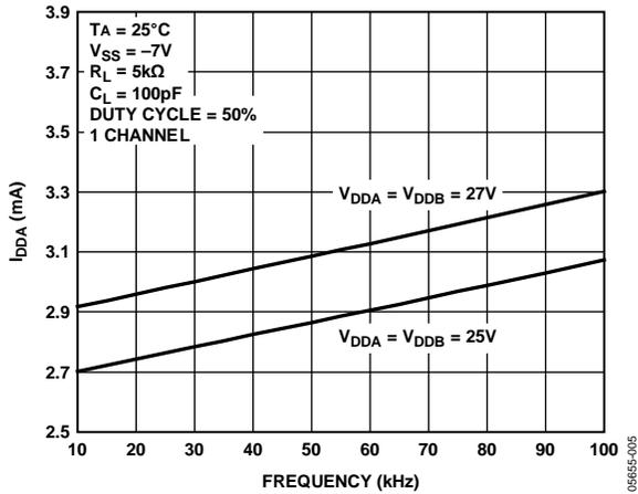
Figure 5. Supply Current ( $I_{DDA}$ ) vs. Frequency
