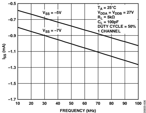
Figure 6. Supply Current ( $I_{SS}$ ) vs. Frequency
