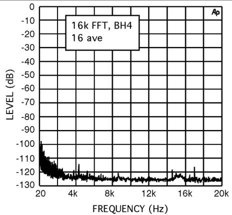
Figure 13. Headphone Amplifier Noise Floor (Analog Loopthrough)
