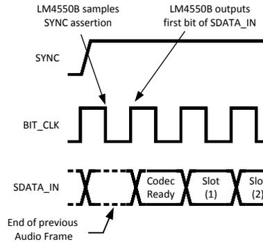
Figure 22. Start of AC Link Input Frame
