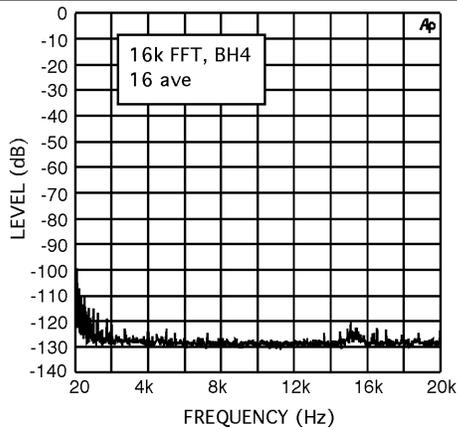
Figure 12. Line Out Noise Floor (Analog Loopthrough)
