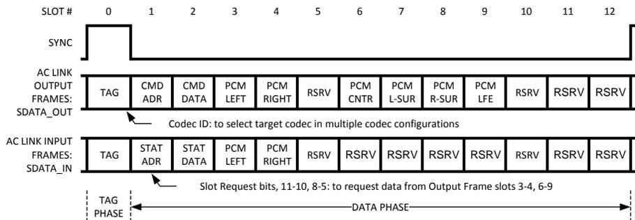
Figure 18. AC Link Bidirectional Audio Frame
