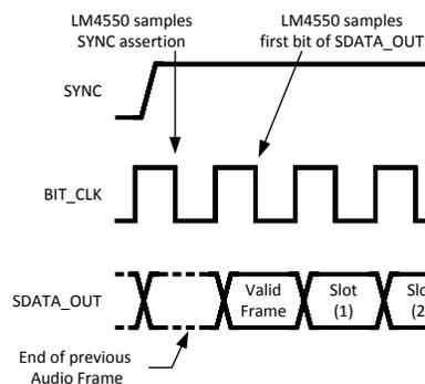
Figure 20. Start of AC Link Output Frame
