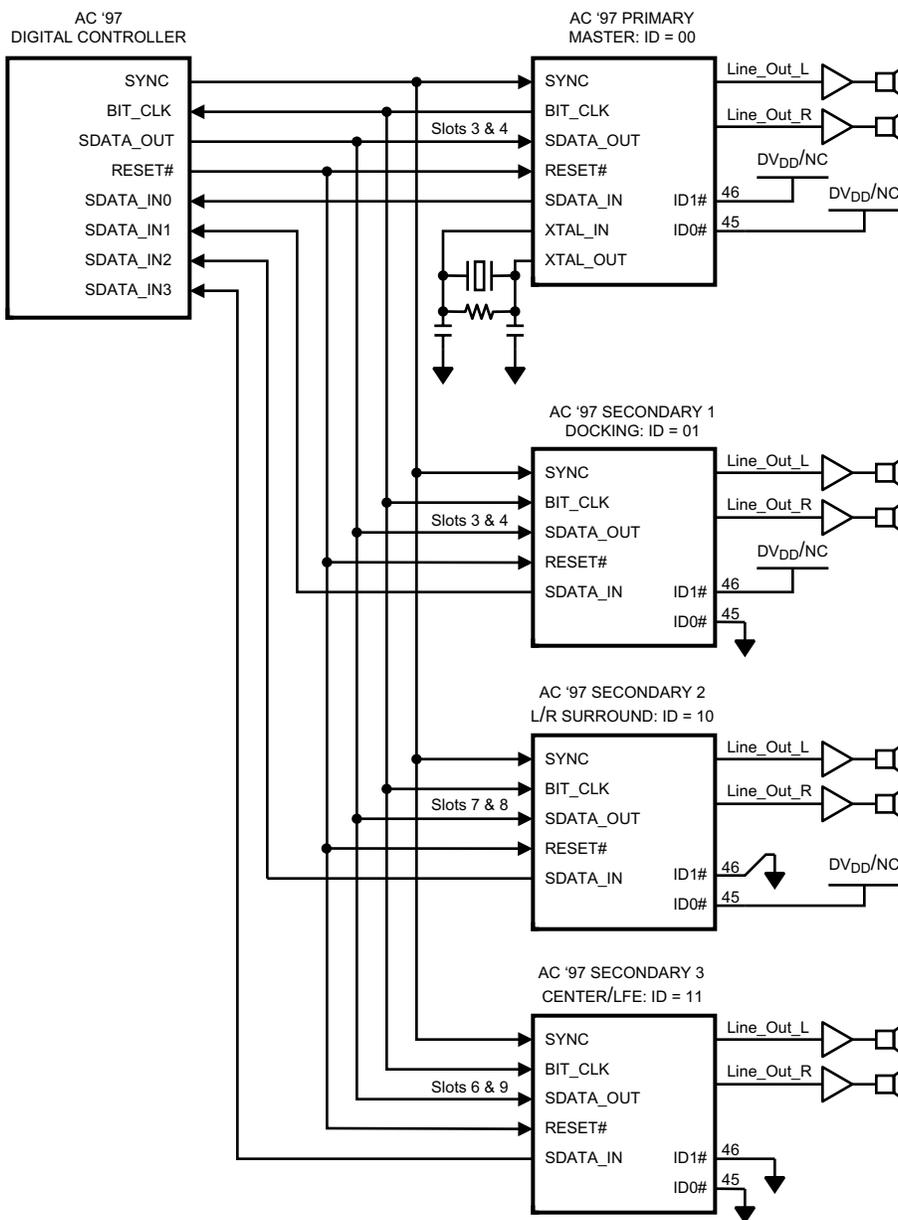
Figure 16. Multiple Codecs using Extended AC Link
