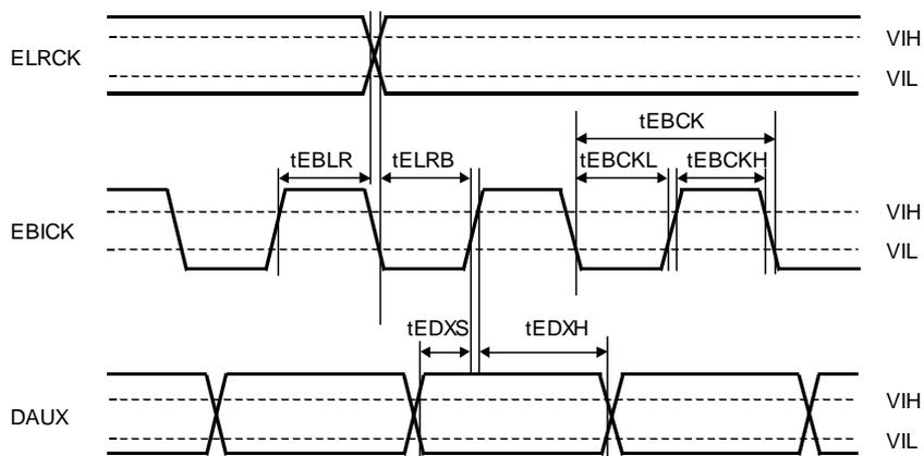
Figure 6. Serial Interface Timing 2 (Slave Mode)
