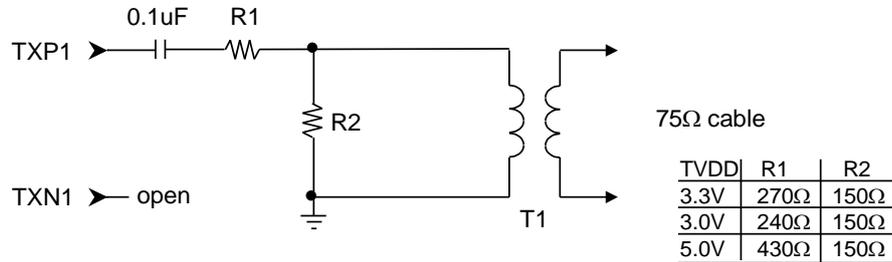
Figure 26. Consumer Output Driver Circuit at AC coupling
