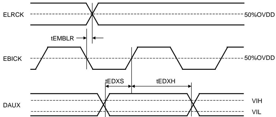
Figure 7. Serial Interface Timing 2 (Master Mode)
