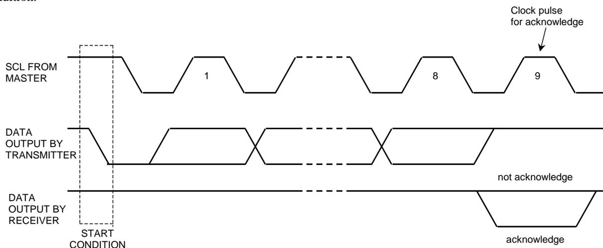
Figure 43. Acknowledge on the I<sup>2</sup>C-bus
