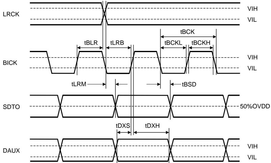
Figure 4. Serial Interface Timing 1 (Slave Mode)
