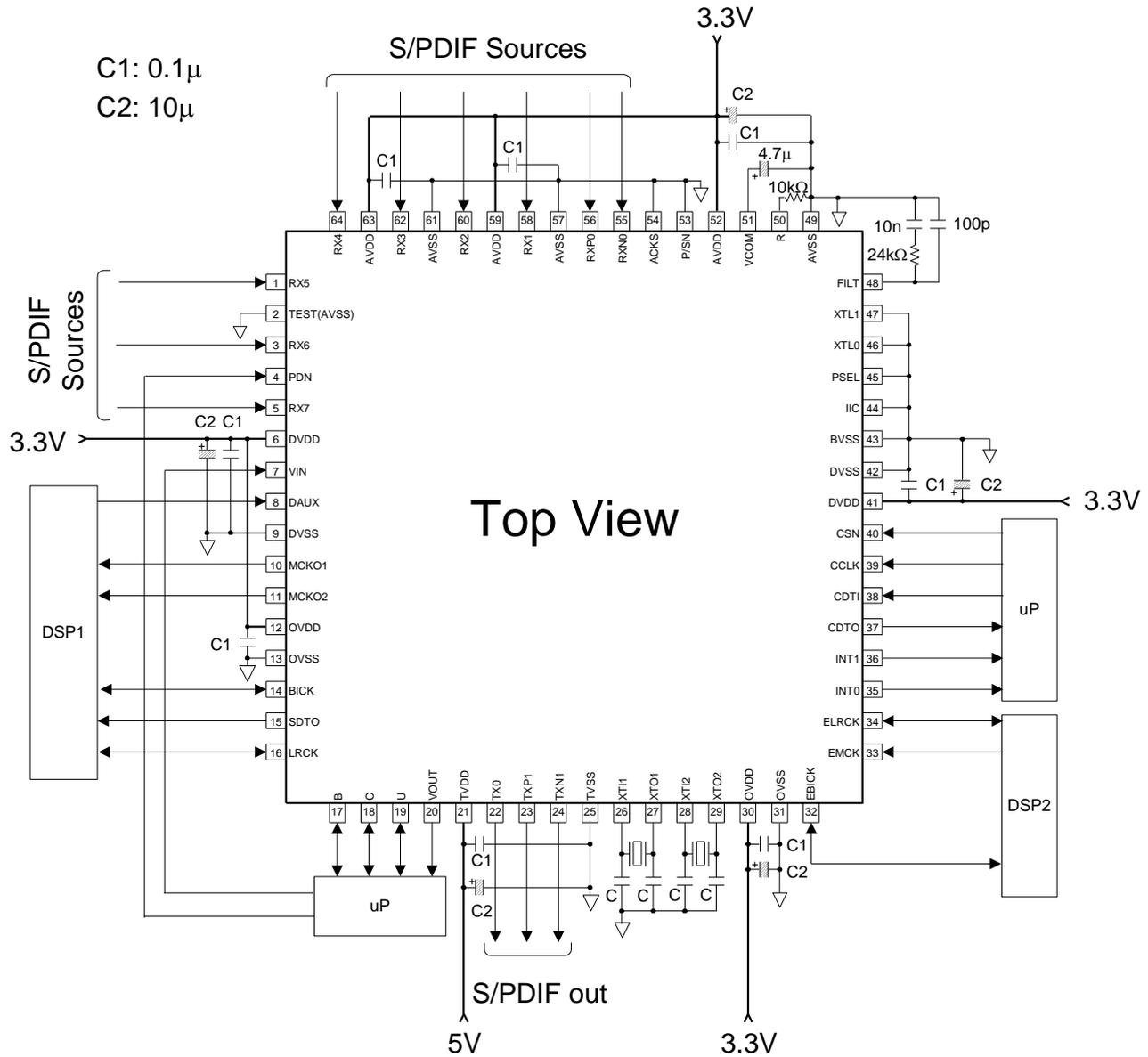
Figure 53. Typical Connection Diagram (4-wire serial mode)
