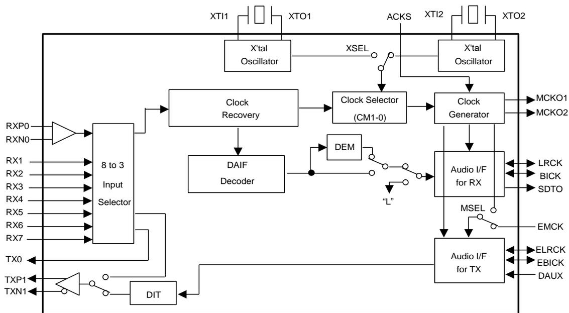
Figure 16. Clocks for DIT/DIR in asynchronous mode
