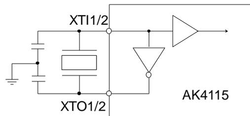
Note: External capacitance depends upon the crystal oscillator (typ. 5-10pF)
