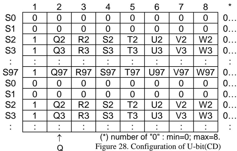
Figure 28. Configuration of U-bit(CD)
