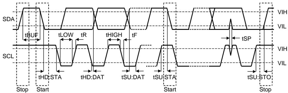
Figure 12. I<sup>2</sup>C Bus mode Timing
