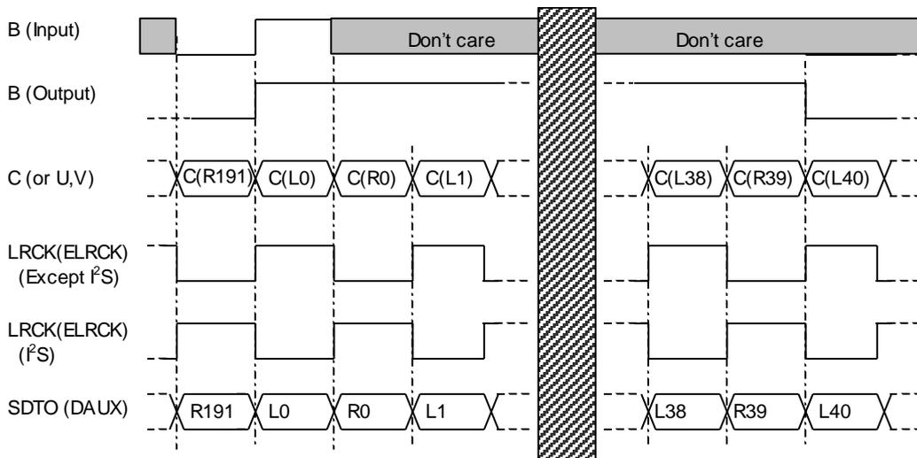
Figure 17. B, C, U, V Input/output timings
