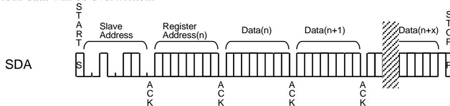
Figure 47. WRITE Operation
