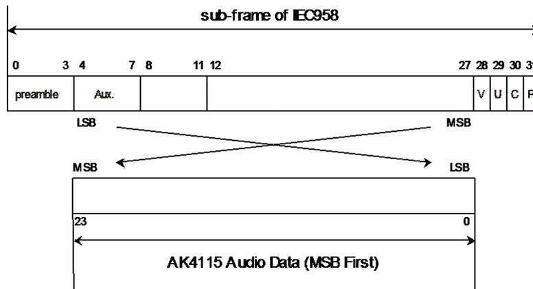
Figure 34. Bit configuration
