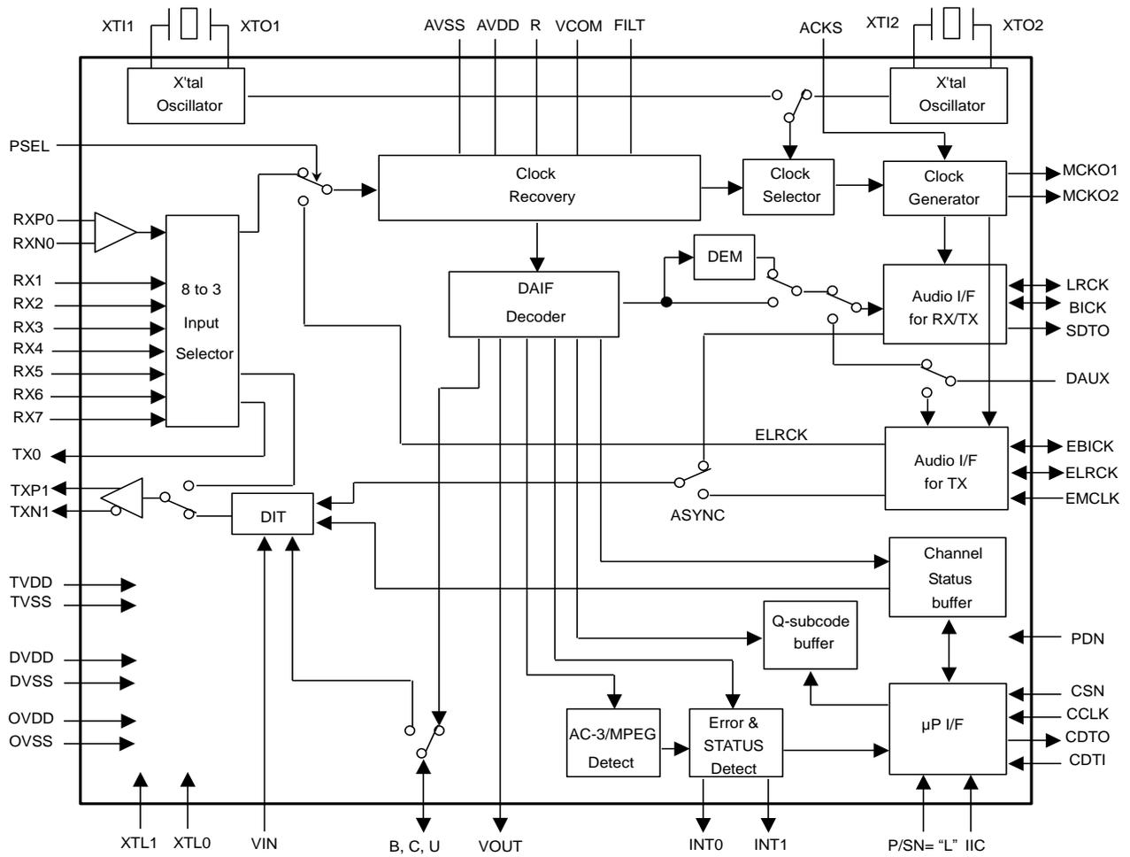
Figure 1. AK4115 Block Diagram in serial mode
