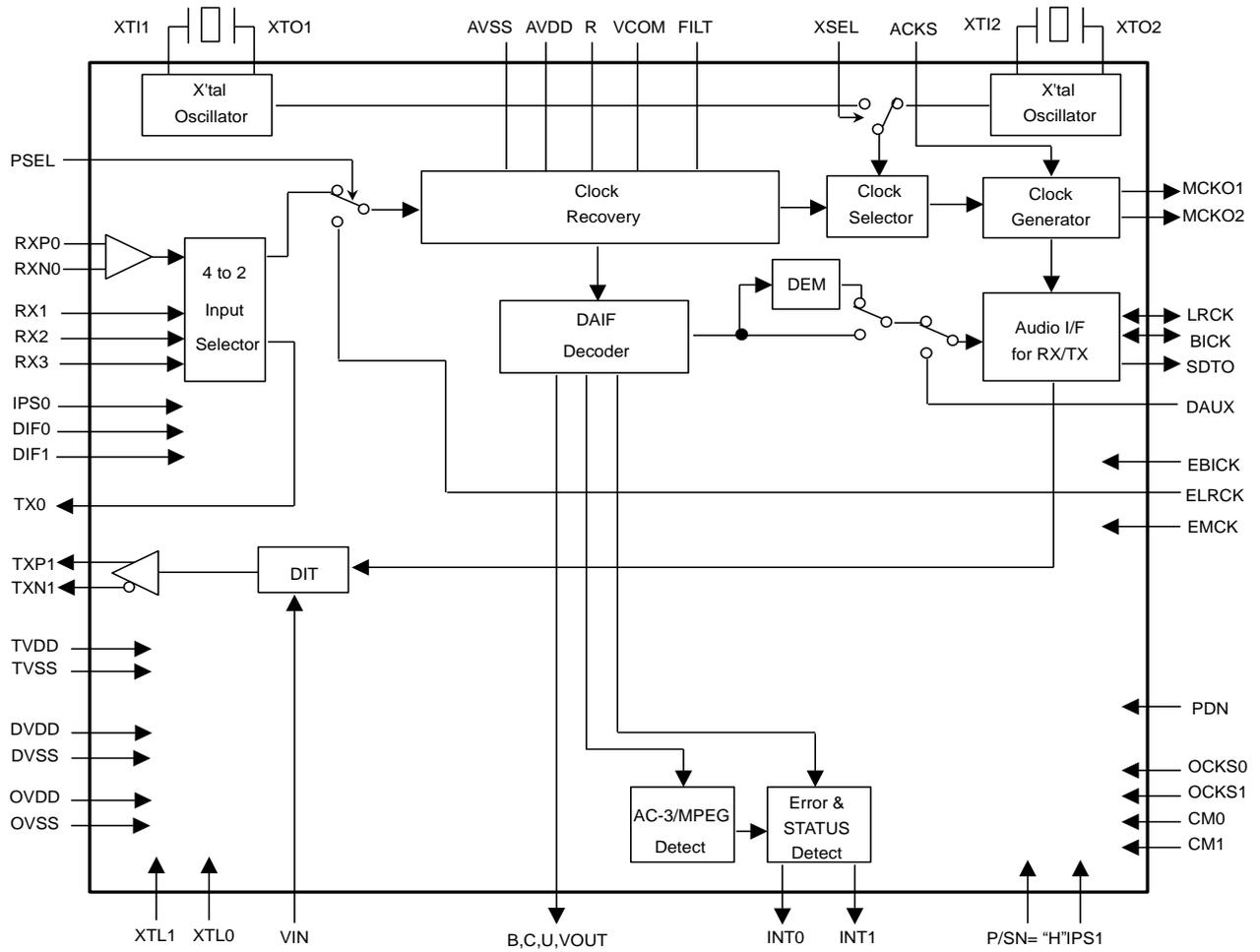
Figure 2. AK4115 Block Diagram in parallel mode
