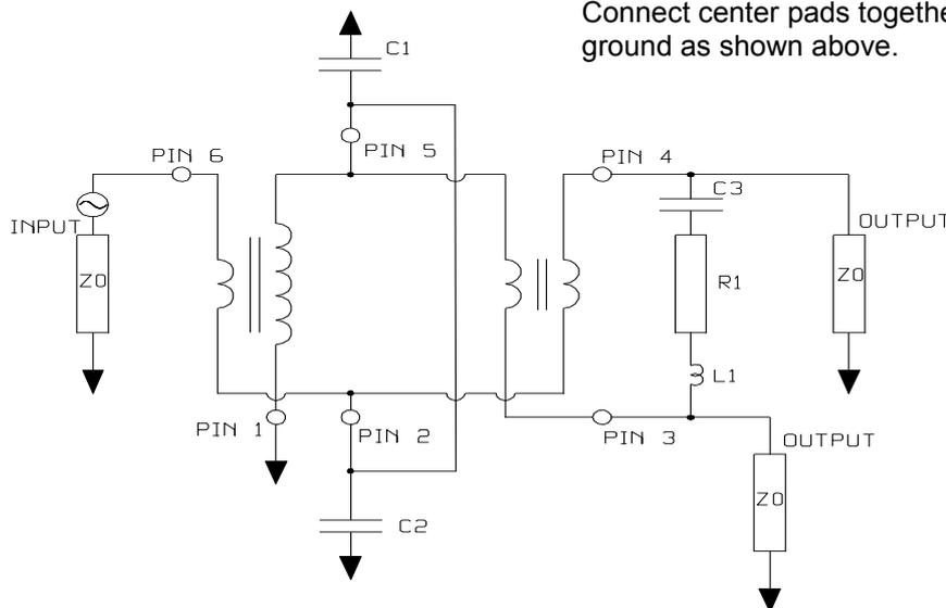
Connect center pads together and isolate them from ground as shown above.
