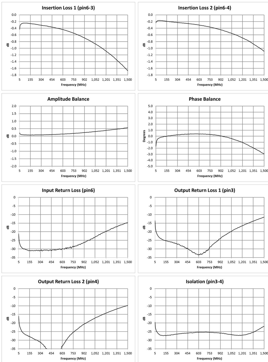
Electrical Specifications:  $T_A = 25^\circ\text{C}$ ,  $Z_0 = 75 \Omega$ ,  $P_{in} = 0\text{dBm}$
