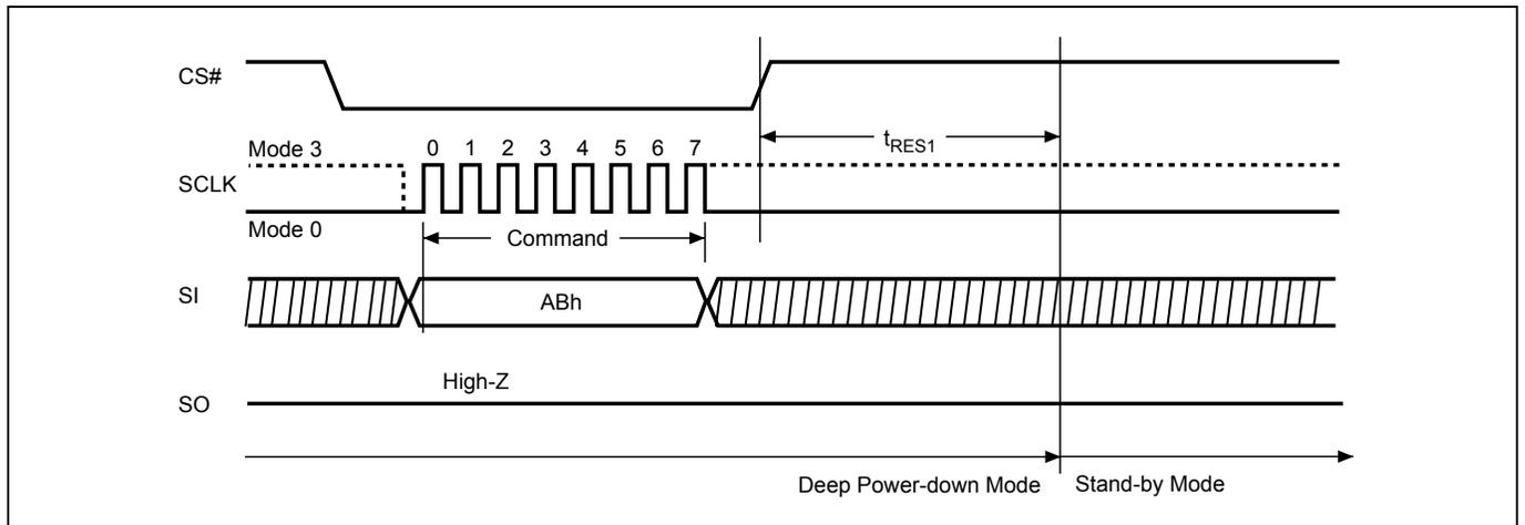
**Figure 23. Release from Deep Power-down (RDP) Sequence (QPI Mode)**
