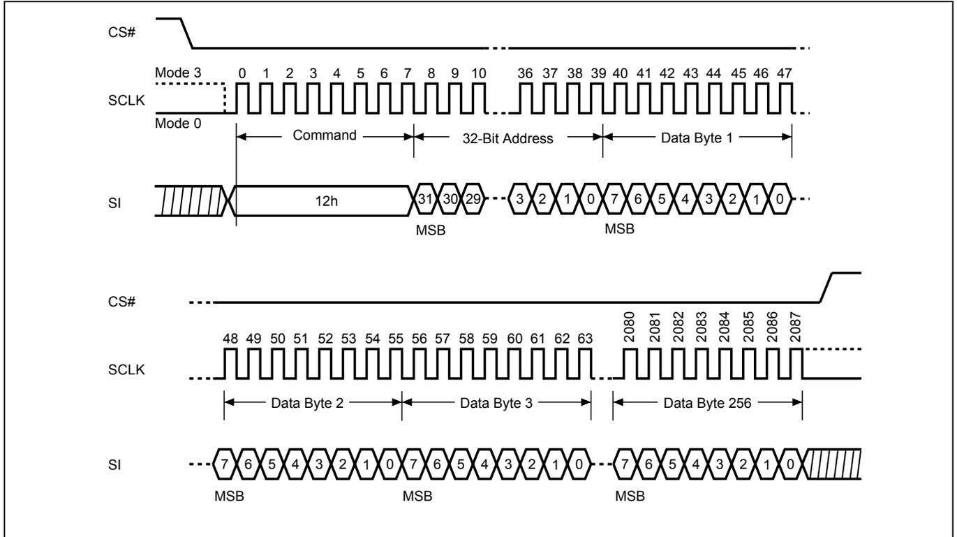
**Figure 68. 4 x I/O Page Program (4PP4B) Sequence (SPI Mode only)**
