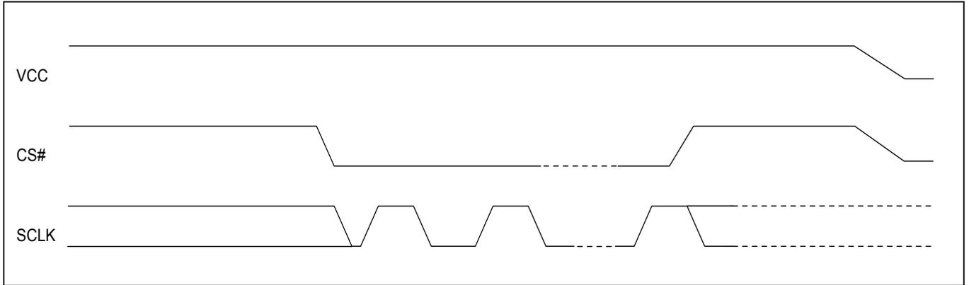
**Figure 126. Power-up Timing**
