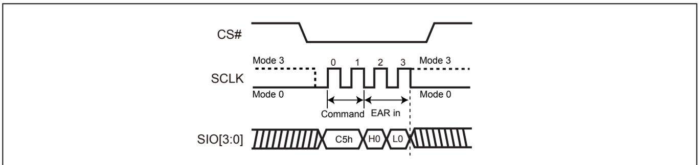
**Figure 9. Read EAR (RDEAR) Sequence (SPI Mode)**
