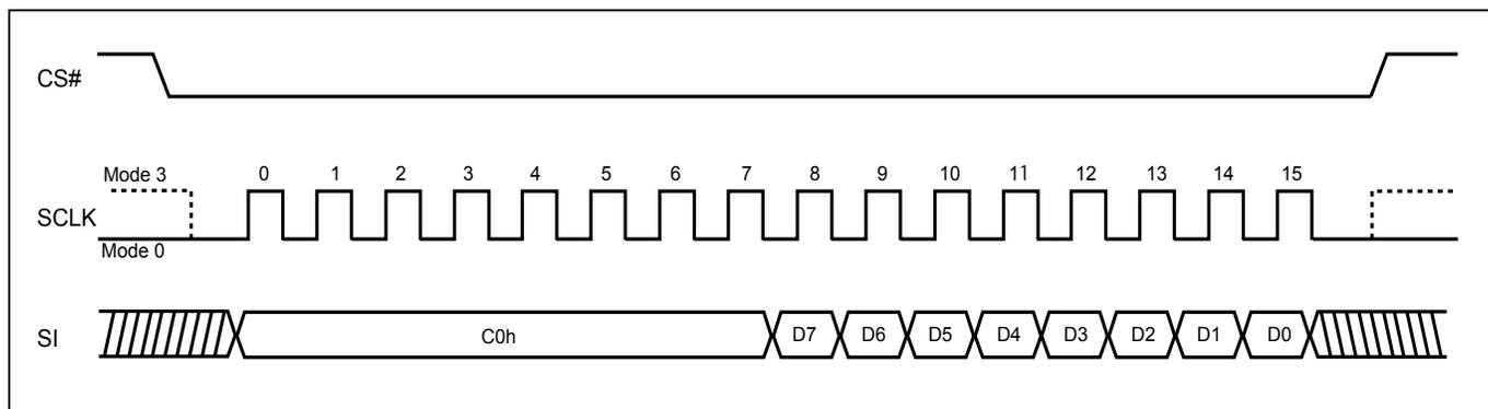
**Figure 74. Burst Read (QPI Mode)**
