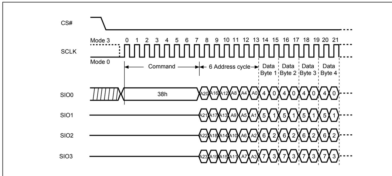
**Note:** Please note the address cycles above are based on 3-byte address mode. For 4-byte address mode, the address cycles will be increased.
