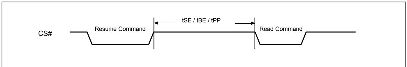
**Figure 113. Resume to Suspend Latency**
