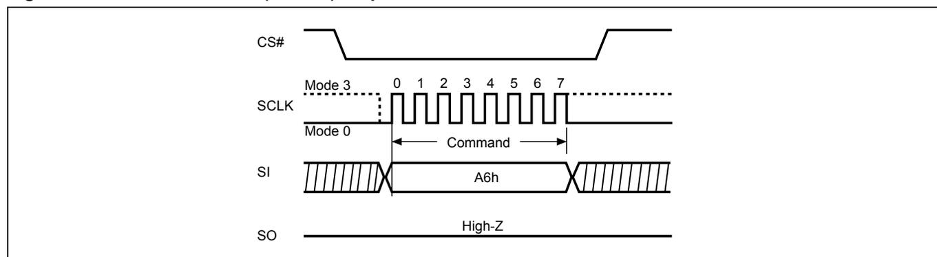
**Figure 102. Read SPB Lock Register (RDSPBLK) Sequence**
