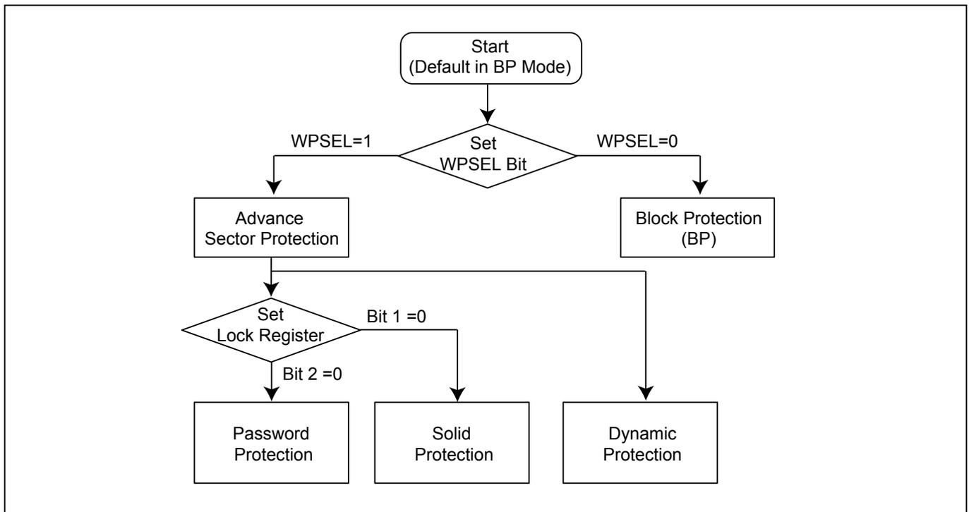
**Figure 97. WPSEL Flow**
