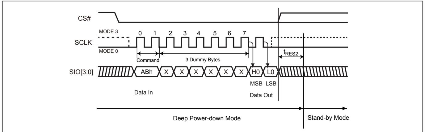
**Figure 22. Release from Deep Power-down (RDP) Sequence (SPI Mode)**
