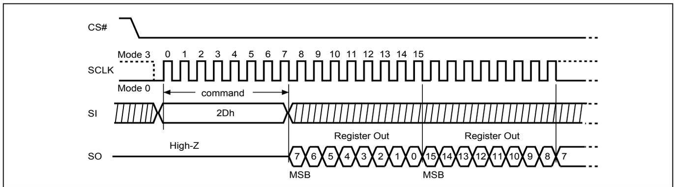
**Figure 100. Write Lock Register (WRLR) Sequence (SPI Mode)**
