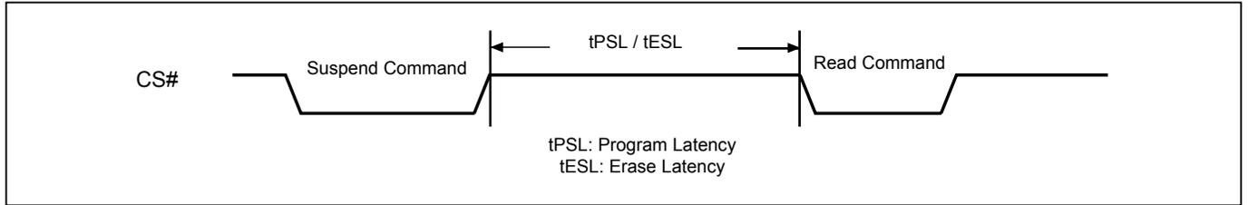
**Figure 112. Resume to Read Latency**
