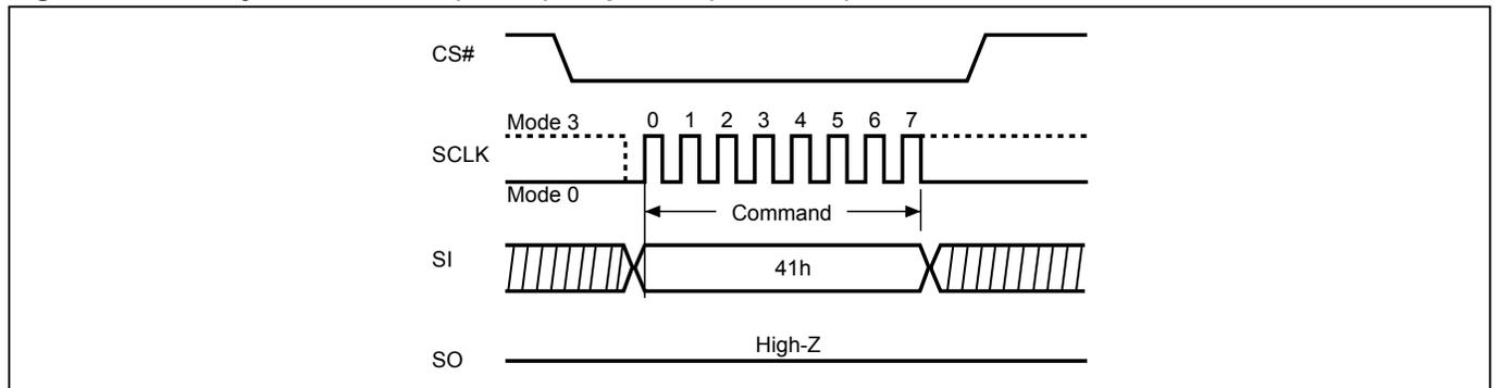
**Figure 18. Factory Mode Enable (FMEN) Sequence (QPI Mode)**
