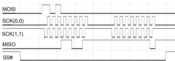
The MAX3420E SPI interface works in modes (0,0) and (1,1) without alteration. The difference is the inactive SCK level. In both modes the data is changed on the SCK falling edge and sampled on the SCK rising edge. Full-duplex mode (FDUPSPI=1) is shown here.
