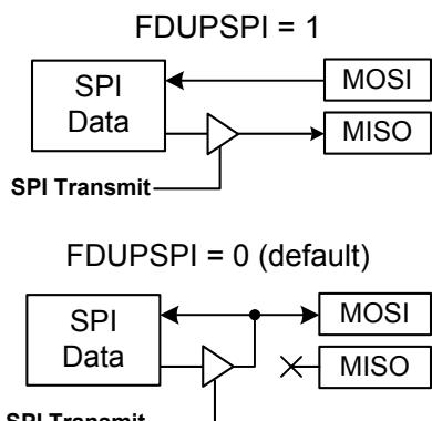
The FDUPSPI bit configures the SPI interface for full-duplex or half-duplex operation. In half-duplex mode (FDUPSPI = 0) the MISO pin can be left unconnected.
