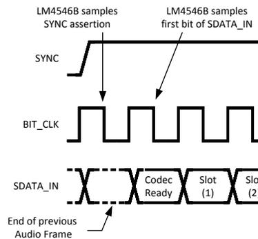
**Figure 16. Start of AC Link Input Frame**
