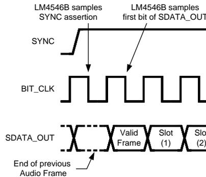
Figure 14. Start of AC Link Output Frame
