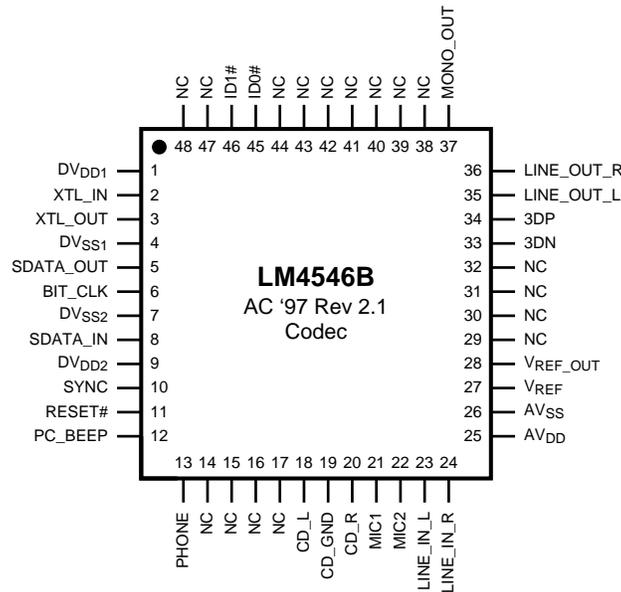
Figure 6. See Package Number PT0048A (Top View)
