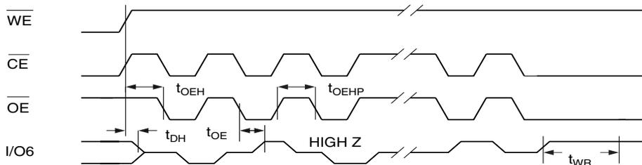
Notes: 1. Toggling either  $\overline{OE}$  or  $\overline{CE}$  or both  $\overline{OE}$  and  $\overline{CE}$  will operate toggle bit. The  $t_{OEHP}$  specification must be met by the toggling input(s).
