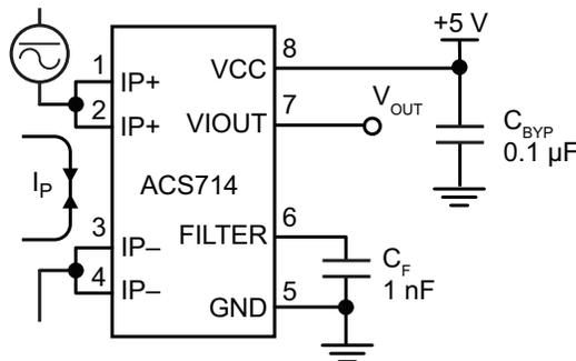
Application 1. The ACS714 outputs an analog signal,  $V_{OUT}$ , that varies linearly with the uni- or bi-directional AC or DC primary sampled current,  $I_p$ , within the range specified.  $C_F$  is recommended for noise management, with values that depend on the application.
