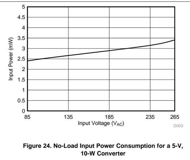
Figure 24. No-Load Input Power Consumption for a 5-V, 10-W Converter
