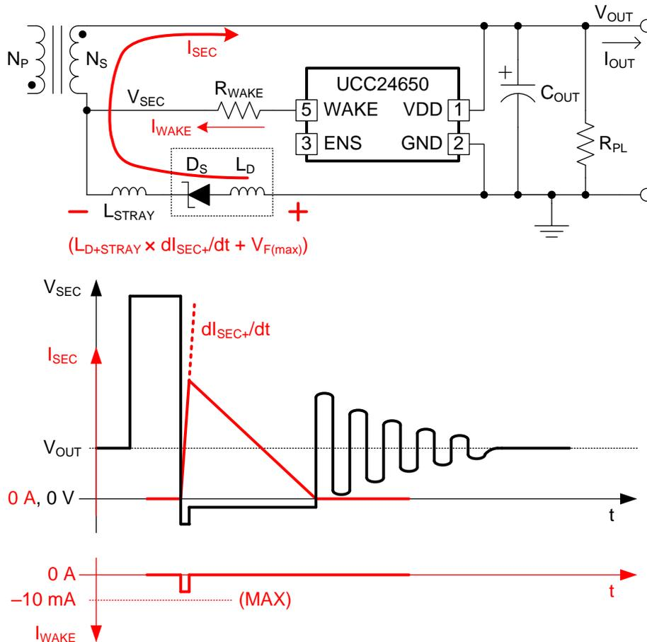
**Figure 16. High  $dI_{SEC}/dt$  may Generate Significant  $I_{WAKE}$ .**
