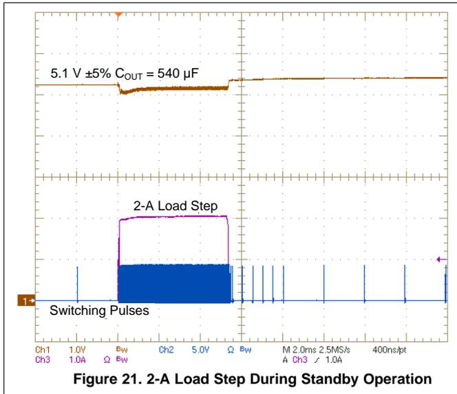
Figure 21. 2-A Load Step During Standby Operation
