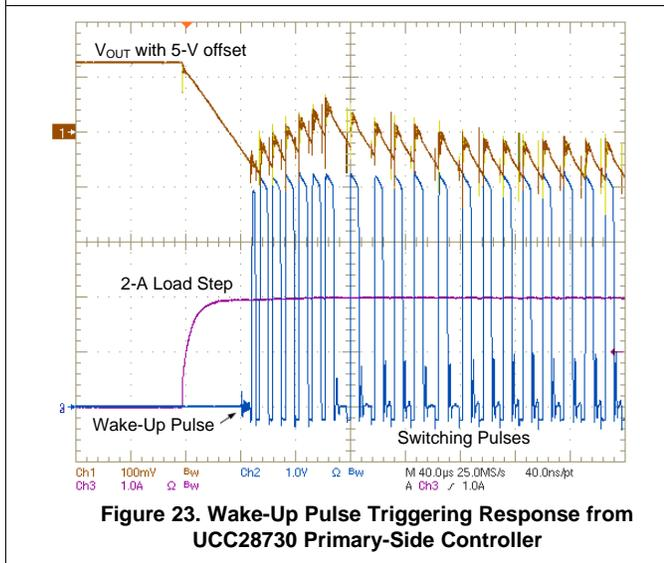
Figure 23. Wake-Up Pulse Triggering Response from UCC28730 Primary-Side Controller
