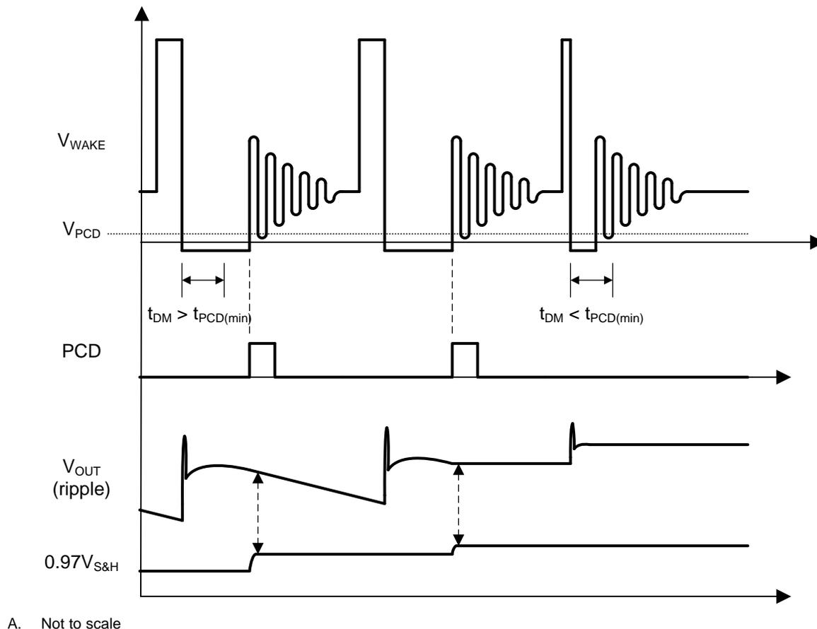
**Figure 11. Timing Diagram of Internal PCD Signal**
