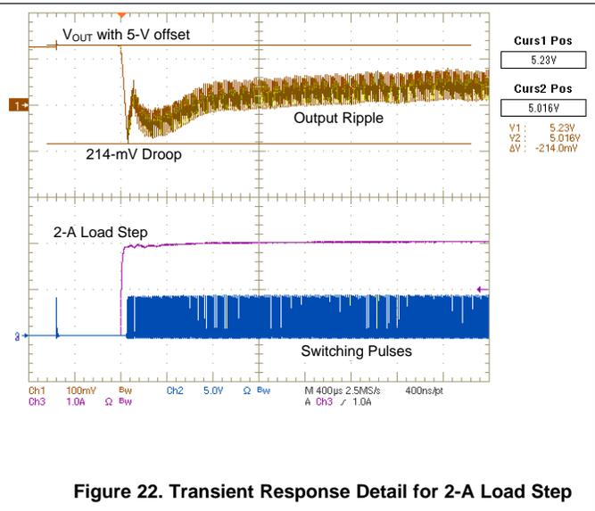
Figure 22. Transient Response Detail for 2-A Load Step
