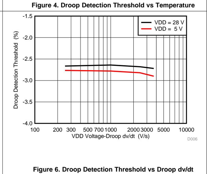
Figure 6. Droop Detection Threshold vs Droop dv/dt
