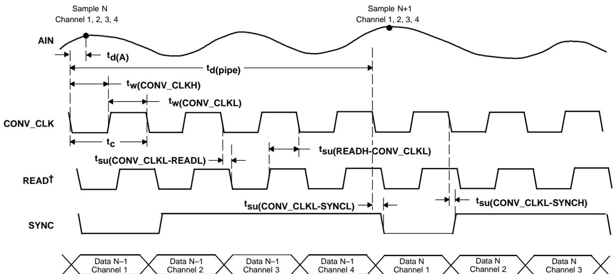
†READ is the logical combination from  $\overline{\text{CS0}}$ , CS1 and  $\overline{\text{RD}}$
