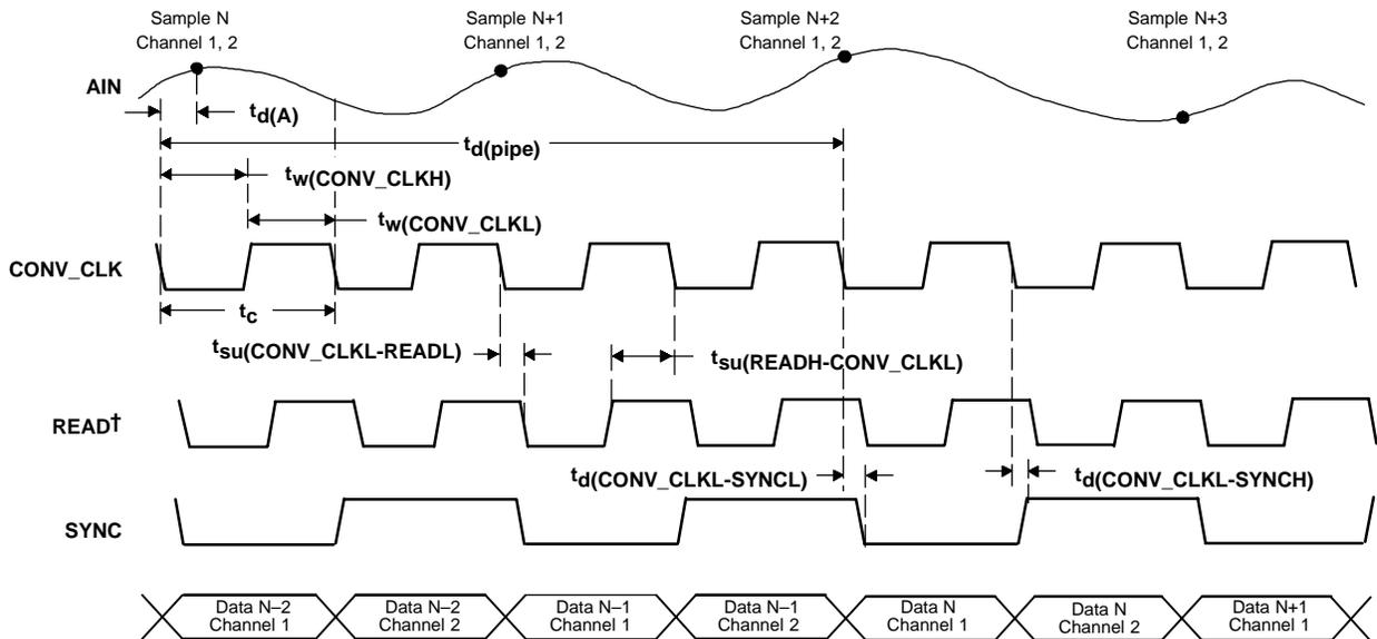
†READ is the logical combination from  $\overline{CS0}$ , CS1 and  $\overline{RD}$
