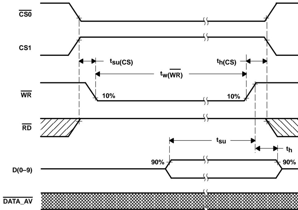
Figure 33. Write Timing Diagram Using  $\overline{WR}$  ( $\overline{WR}$ -controlled)
