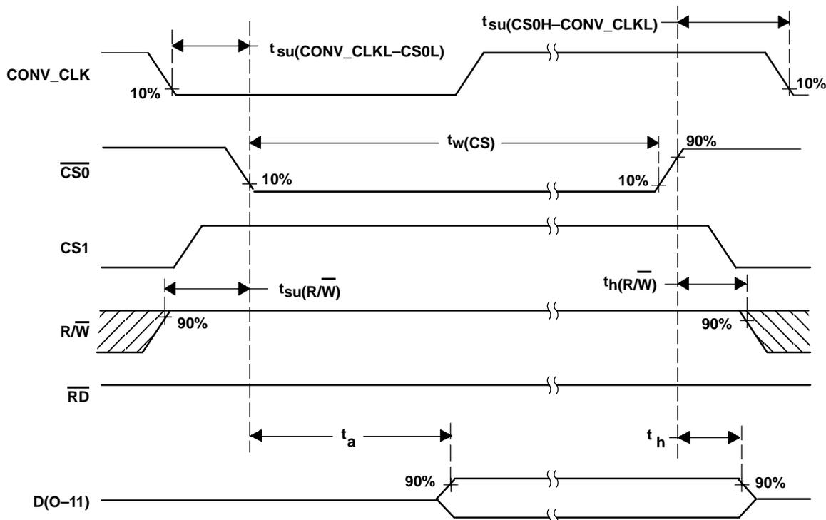
Figure 34. Read Timing Diagram Using  $\overline{R/\overline{W}}$  ( $\overline{CS0}$ -controlled)
