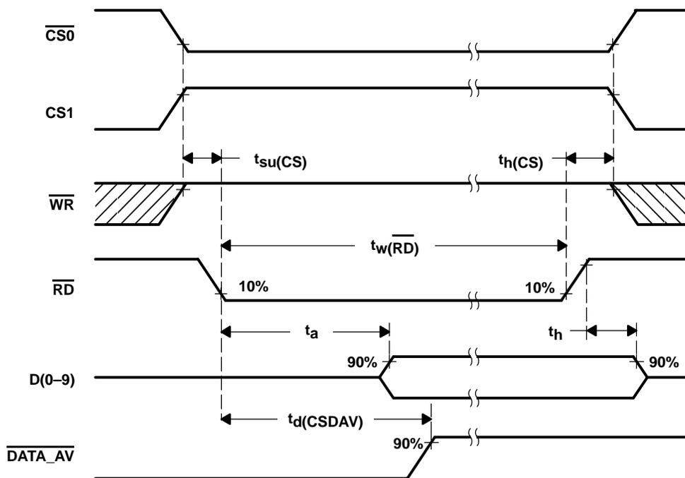
**Figure 32. Read Timing Diagram Using  $\overline{RD}$  ( $\overline{RD}$ -controlled)**
