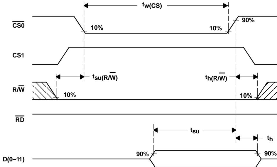
Figure 35. Write Timing Diagram Using  $\overline{R/W}$  ( $\overline{CS0}$ -controlled)
