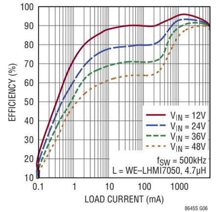
LT8645S Low Load Efficiency at 3.3V<sub>OUT</sub>
