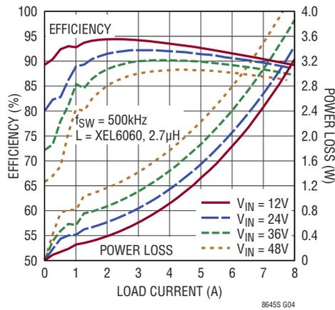
LT8645S Low Load Efficiency at 5V<sub>OUT</sub>
