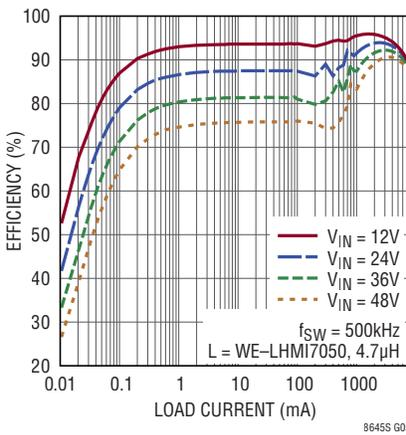
LT8646S Low Load Efficiency at 5V<sub>OUT</sub>
