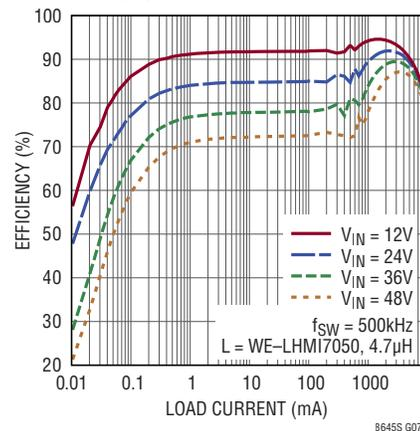
LT8646S Low Load Efficiency at 3.3V<sub>OUT</sub>
