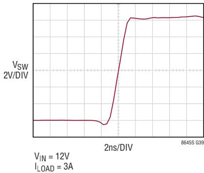
Switching Waveforms, Full Frequency Continuous Operation
