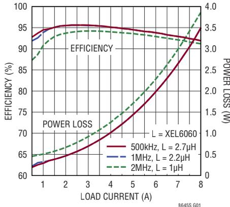
12V<sub>IN</sub> to 3.3V<sub>OUT</sub> Efficiency vs Frequency
