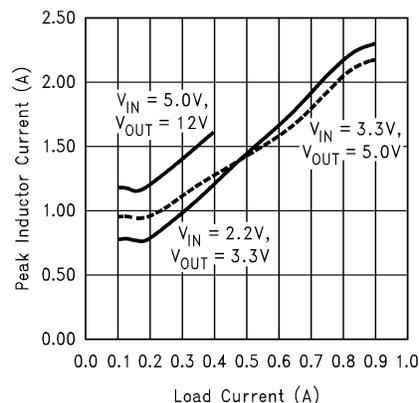
**Figure 16. Peak Inductor Current vs Load Current**
