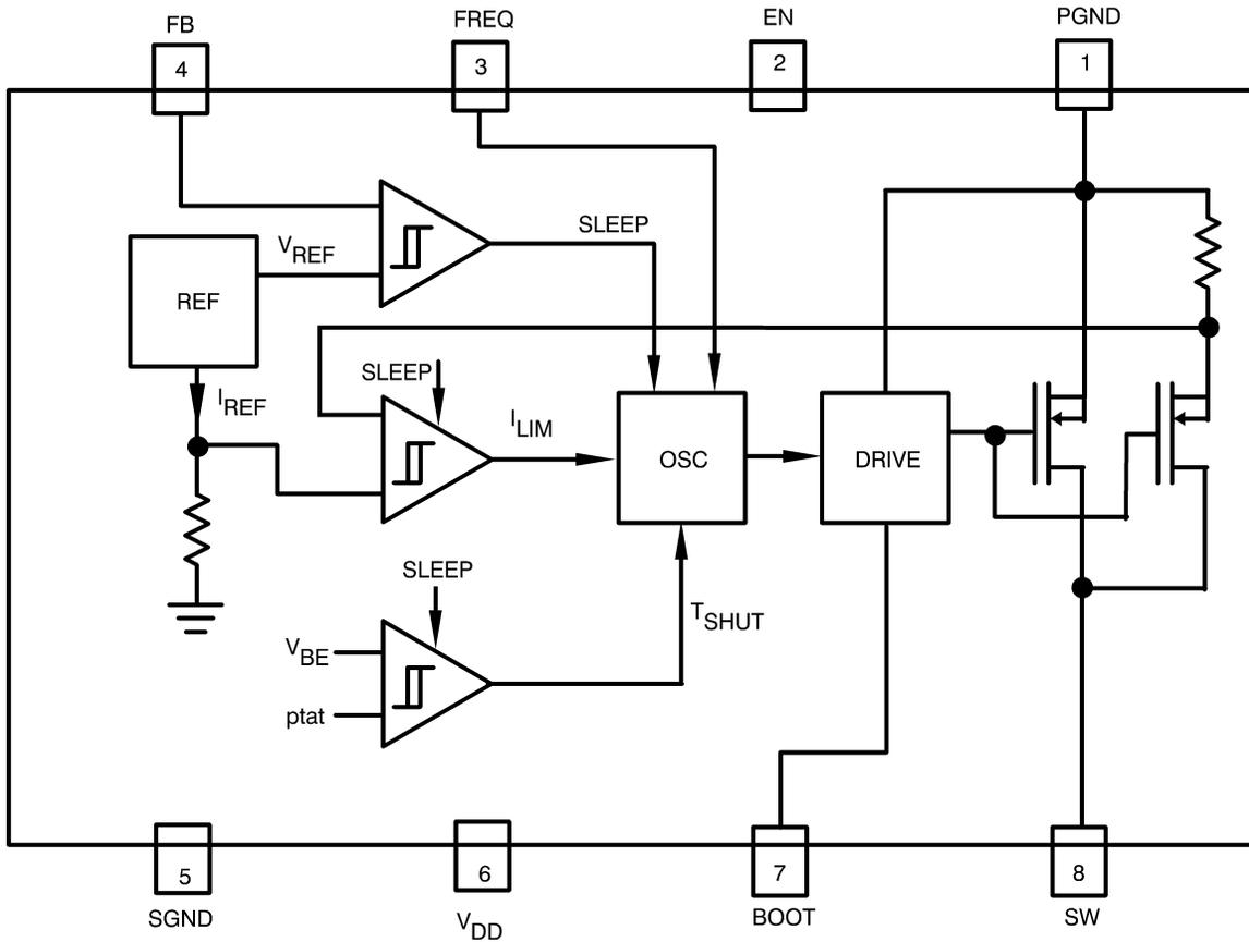
Figure 13. Block Diagram
