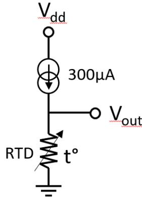
$$V_{out} = R_{RTD} \times I_{cc}$$
