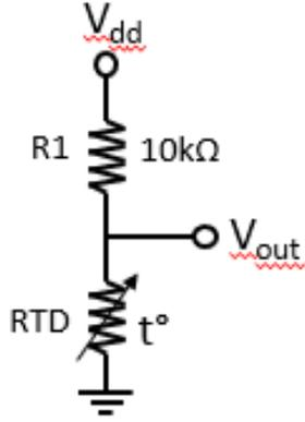
$$V_{out} = \frac{R_{RTD} \times V_{dd}}{(R1 + R_{RTD})}$$
