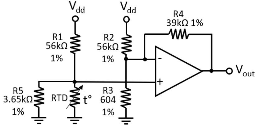
$$V_{out} = \frac{\left[ \frac{R_{RTD} \times R5}{R_{RTD} + R5} \right] \times V_{dd}}{R1 + \left[ \frac{R_{RTD} \times R5}{R_{RTD} + R5} \right]} \times \left[ 1 + R4 \times \left[ \frac{1}{R2} + \frac{1}{R3} \right] \right] - \frac{R4 \times V_{dd}}{R2}$$
