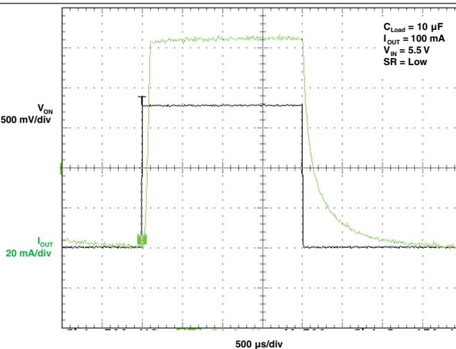
Figure 23.  $t_{ON}$  Response
