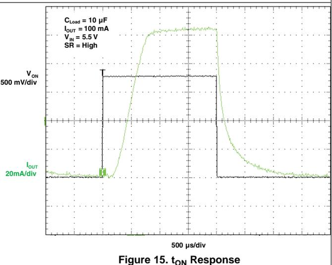
Figure 15.  $t_{ON}$  Response
