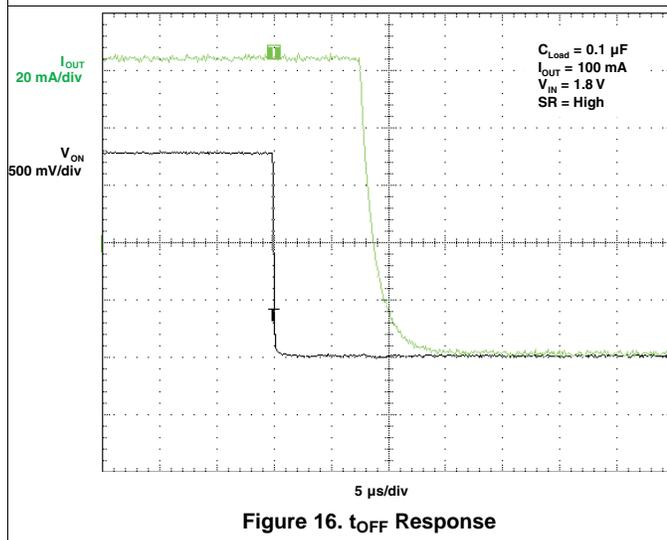
Figure 16.  $t_{OFF}$  Response
