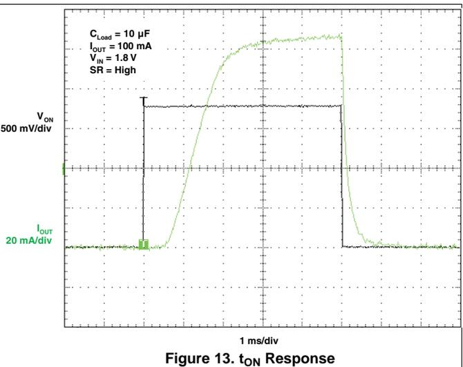
Figure 13.  $t_{ON}$  Response
