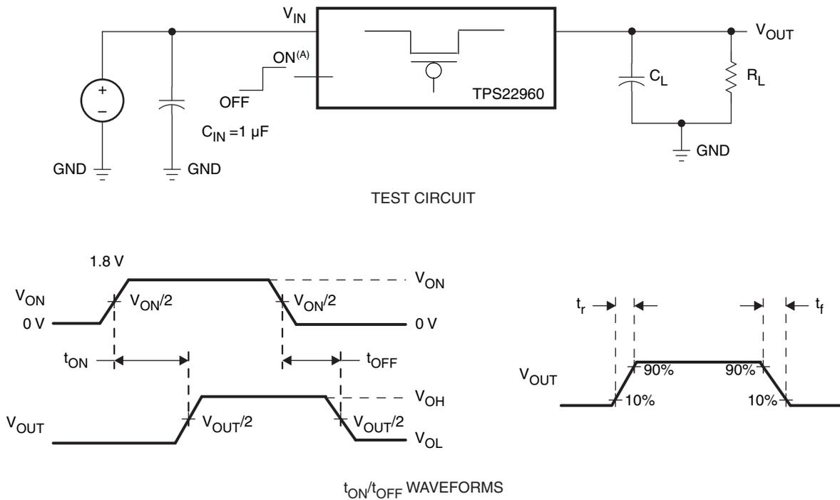
A.  $t_{rise}$  and  $t_{fall}$  of the control signal is 100 ns.
