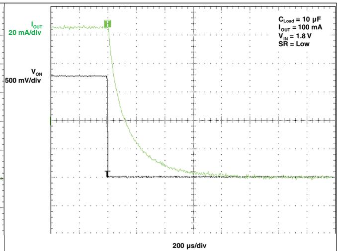
Figure 25.  $t_{OFF}$  Response
