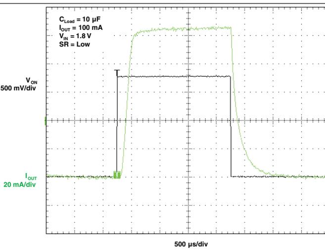
Figure 21.  $t_{ON}$  Response
