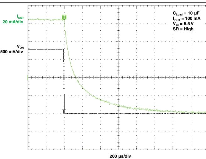
Figure 19.  $t_{OFF}$  Response
