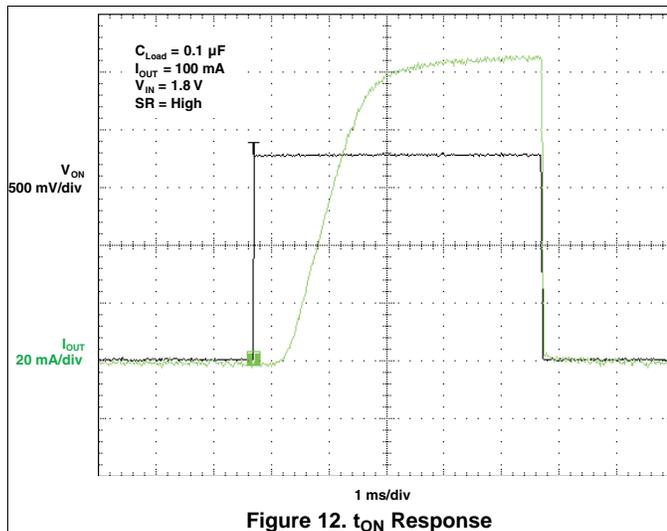
Figure 12.  $t_{ON}$  Response
