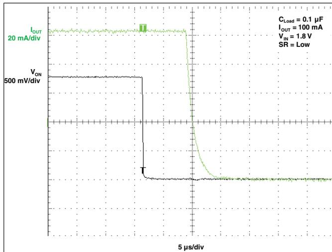
Figure 24.  $t_{OFF}$  Response
