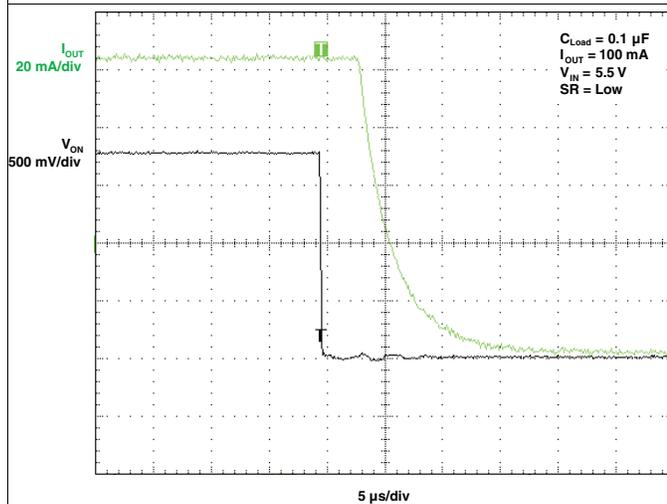
Figure 26.  $t_{OFF}$  Response
