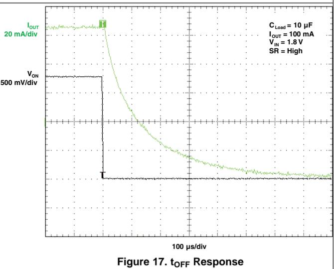
Figure 17.  $t_{OFF}$  Response
