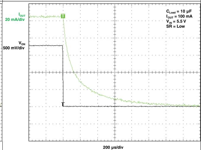
Figure 27.  $t_{OFF}$  Response
