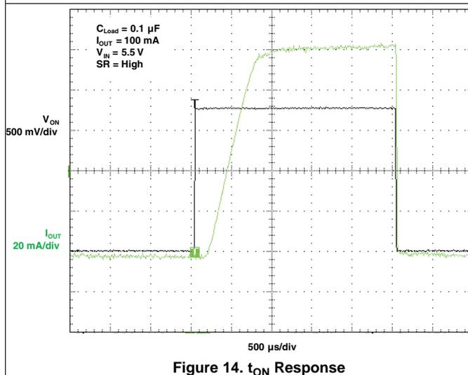
Figure 14.  $t_{ON}$  Response
