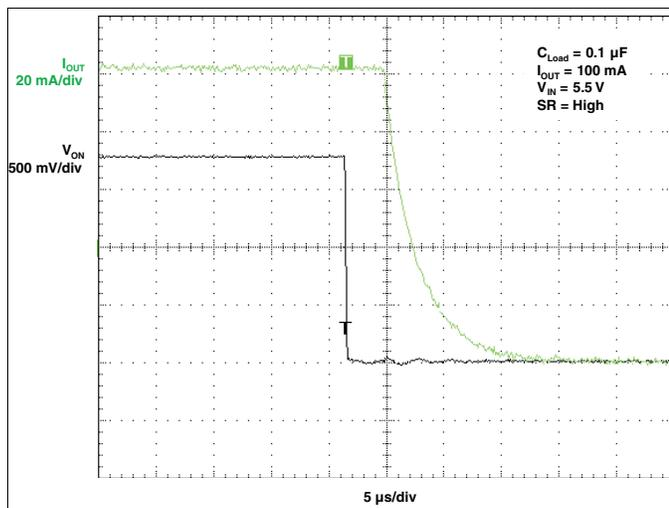
Figure 18.  $t_{OFF}$  Response
