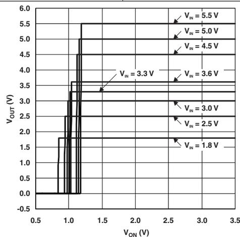
Figure 5. ON Threshold
