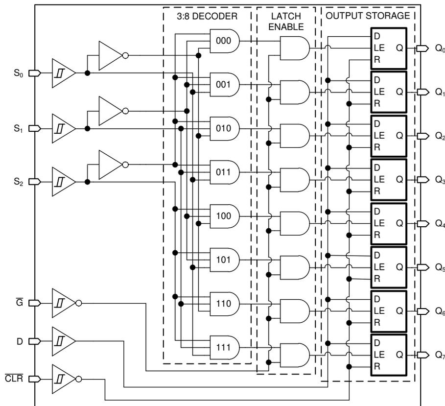
Figure 8-1. Logic Diagram (Positive Logic) for SN74HCS259
