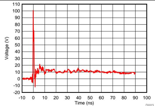
Figure 4. 8-kV IEC 61000-4-2 Clamping Voltage Waveform, IO pin to GND
