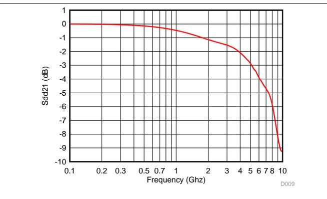
**Figure 10. Differential Insertion Loss**
