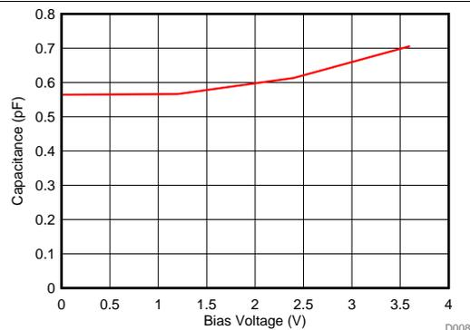
Figure 6. Capacitance vs Bias Voltage
