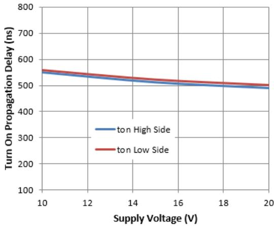
**Figure 4.** Turn-on Propagation Delay vs. Supply Voltage
