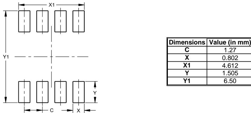
Note : For high voltage applications, the appropriate industry sector guidelines should be considered with regards to creepage and clearance distances between device Terminals and PCB tracking.
