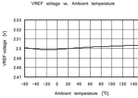
Fig.1 VREF voltage – Ambient temperature
