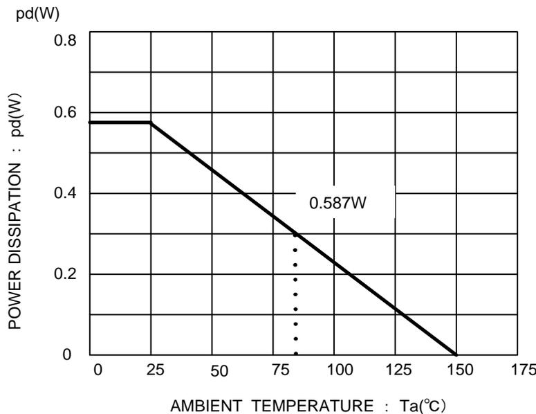
IC mounted on a ROHM standard board (70mm x 70mm x 1.6mm, glass epoxy)
