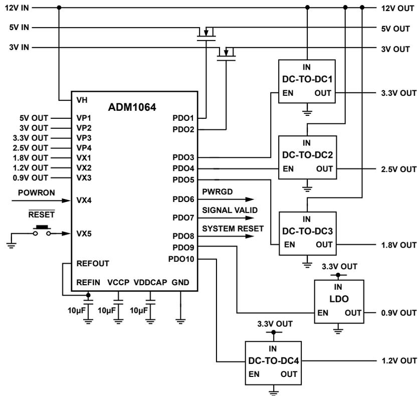
Figure 29. Applications Diagram
