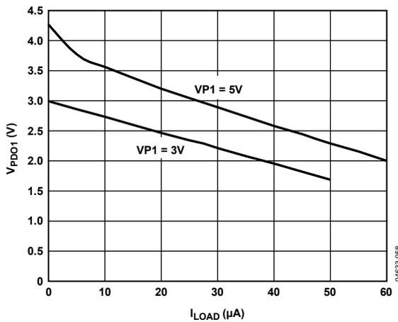
Figure 13.  $V_{PDO1}$  (Weak Pull-Up to  $VPx$ ) vs.  $I_{LOAD}$
