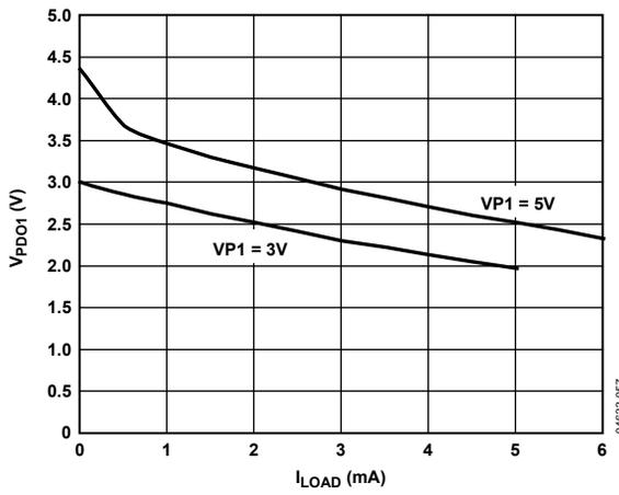
Figure 12.  $V_{PDO1}$  (Strong Pull-Up to  $VPx$ ) vs.  $I_{LOAD}$
