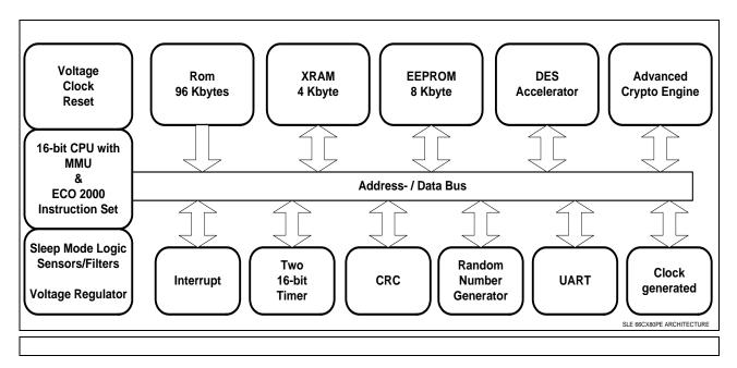
Figure 2: Block Diagram SLE 66CX80PE
