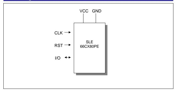
Figure 1: Pin Configuration
