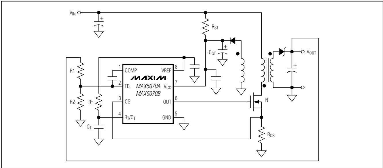
Figure 6. MAX5070A/MAX5070B Typical Application Circuit (Non-Isolated Flyback)
