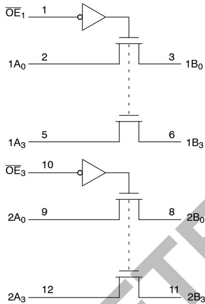
Figure 2. Logic Diagram
