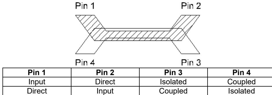
Note: The direct port has a DC connection to the input port and the coupled port has a DC connection to the isolated port.
