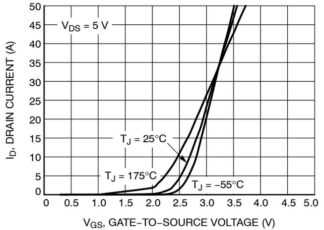
Figure 2. Transfer Characteristics
