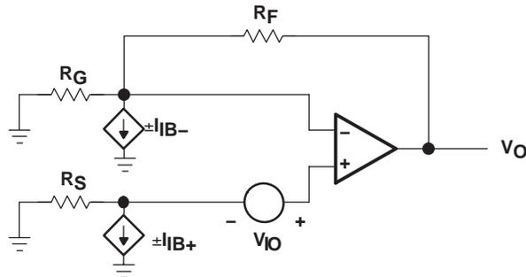
$$V_{OO} = V_{IO} \left( 1 + \frac{R_F}{R_G} \right) \pm I_{IB+} R_S \left( 1 + \frac{R_F}{R_G} \right) \pm I_{IB-} R_F$$
