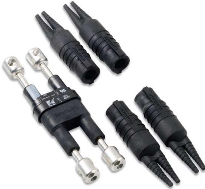
LEX-YY-S and LEX-YYC-S series breakaway fuseholders meet state and federal highway commission safety standards requiring fuseholders to readily disconnect from power in case of a pole knockdown. The breakaway feature consists of a receptacle permanently attached to the power line and a fuseholder with matching terminals. If a knockdown occurs, the parts separate leaving the energized conductor recessed and unexposed.
