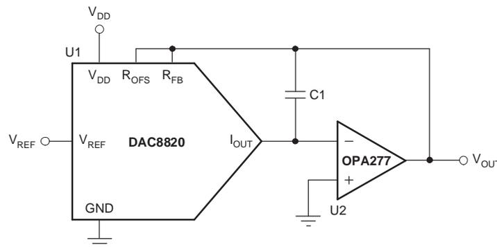
Figure 41. Gain Peaking Prevention Circuit with Compensation Capacitor
