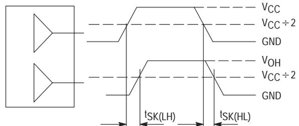
Figure 10. Output-to-output Skew  $t_{SK(O)}$
