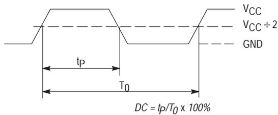
Figure 9. Output Duty Cycle (DC)
