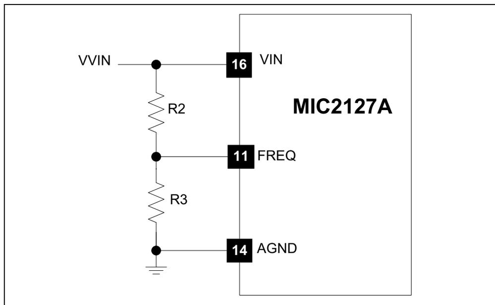
**FIGURE 2-2:** Switching Frequency Adjustment.
