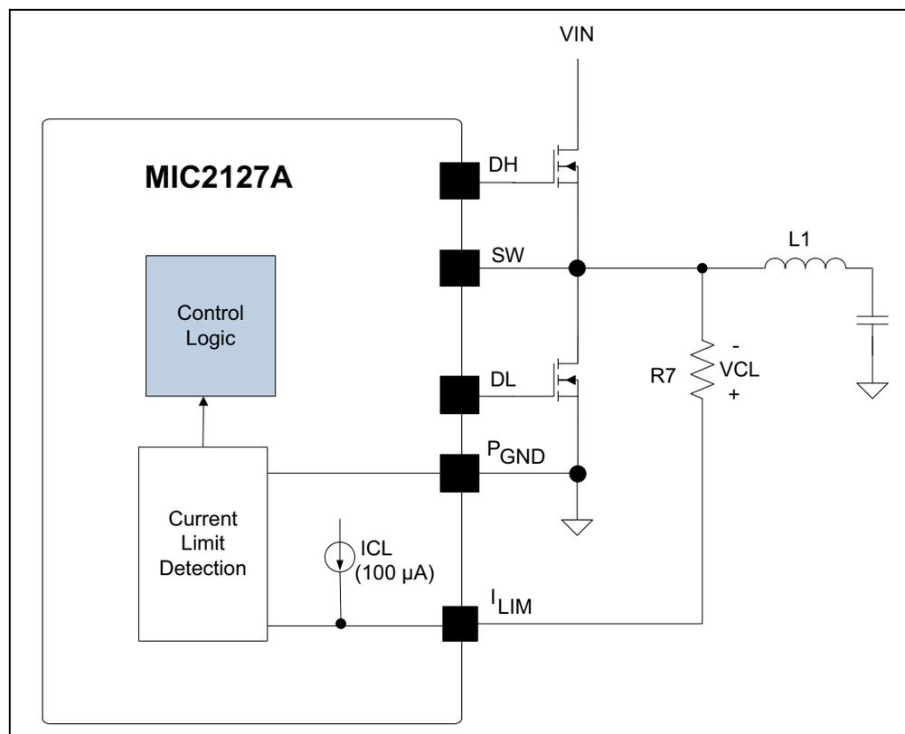
**FIGURE 2-1:** Switching Frequency Adjustment.
