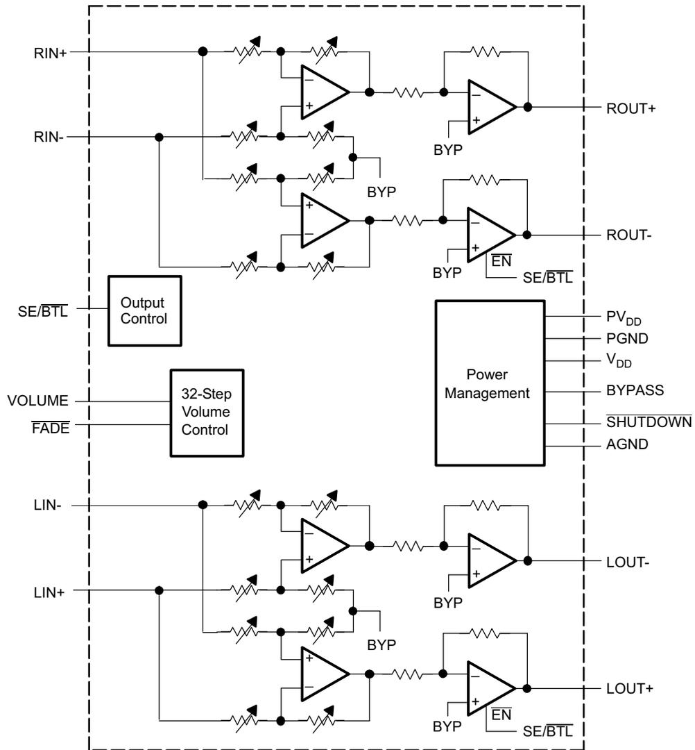
NOTE: All resistor wipers are adjusted with 32 step volume control.
