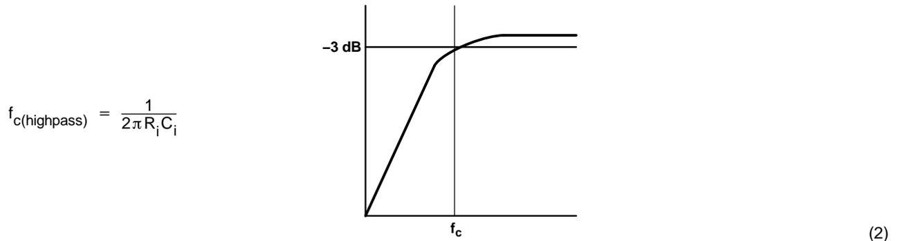
The value of C<sub>i</sub> is important to consider as it directly affects the bass (low frequency) performance of the circuit. Consider the example where R<sub>i</sub> is 70 kΩ and the specification calls for a flat-bass response down to 40 Hz. [Equation 2](#) is reconfigured as [Equation 3](#).
