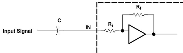
Figure 25. Resistor on Input for Cut-Off Frequency
