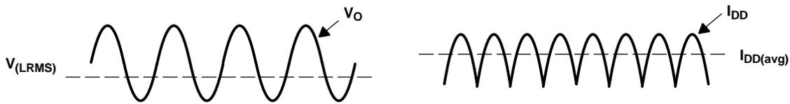
Figure 28. Voltage and Current Waveforms for BTL Amplifiers
