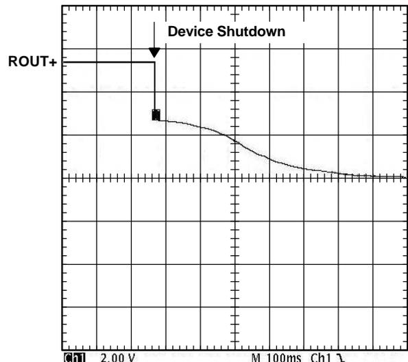
Figure 23. Shutdown Sequence in the Fade-off Mode
