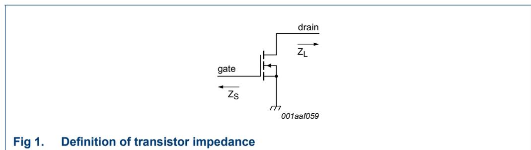
**Fig 1. Definition of transistor impedance**
