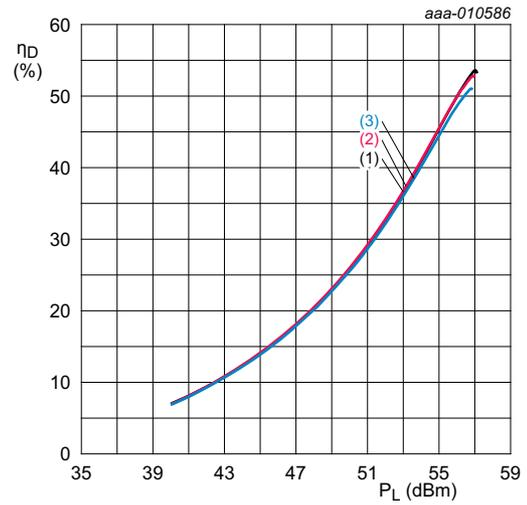
$V_{DS} = 28\text{ V}; I_{Dq} = 3400\text{ mA}; t_p = 100\text{ }\mu\text{s}; \delta = 10\text{ \%}.$
