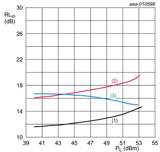
$V_{DS} = 28\text{ V}; I_{Dq} = 3400\text{ mA}.$
