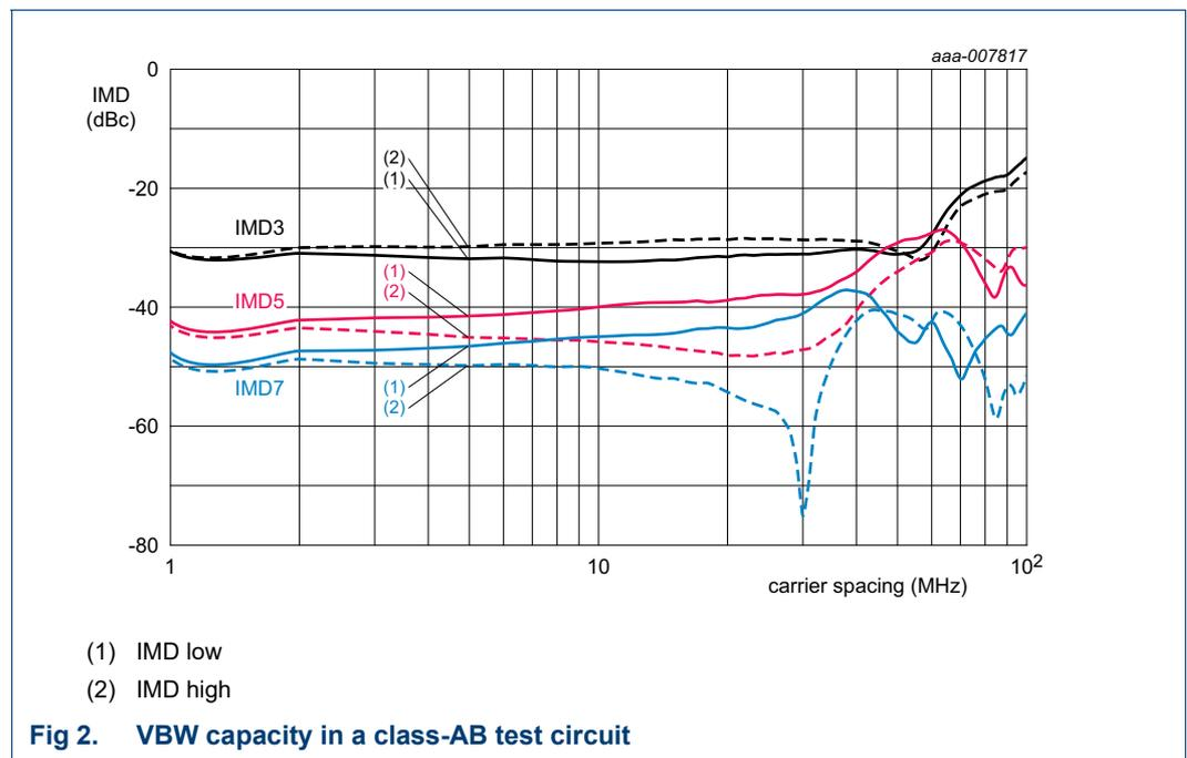
**Fig 2. VBW capacity in a class-AB test circuit**
