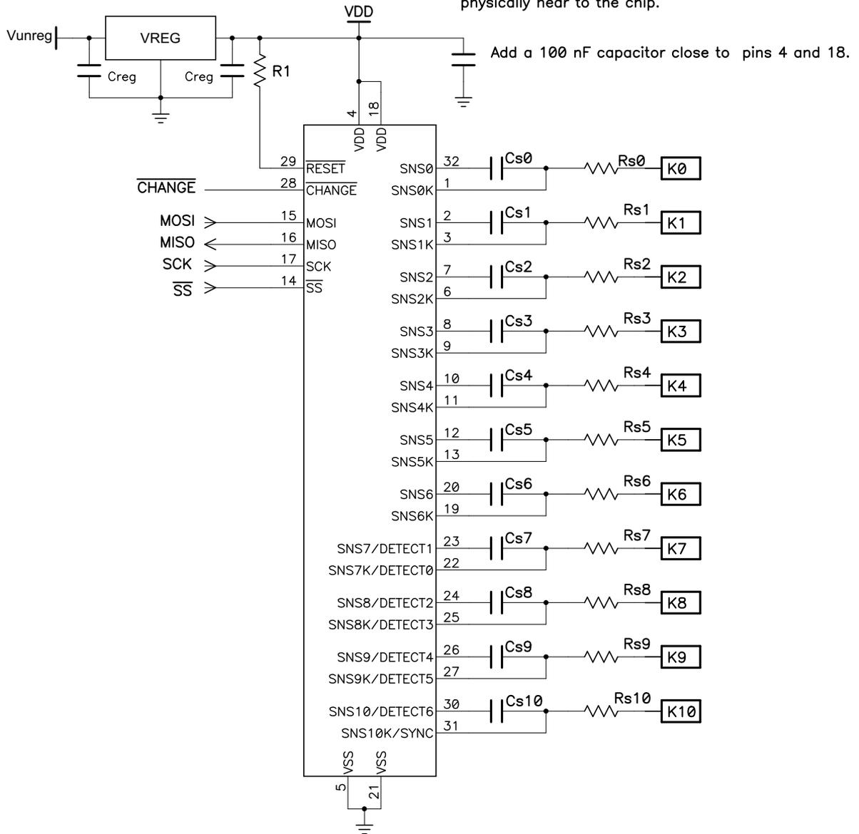
**Figure 1-3. Typical Circuit: 10 Keys With External Trigger (SYNC Mode)**
